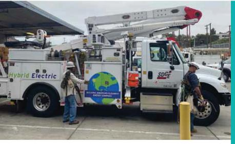
SDG&E uses a fleet of cleaner and quieter hybrid bucket trucks to repair overhead power lines. Unlike conventional bucket trucks, these do not produce loud noises or fumes. Auxiliary functions, such as the bucket and crane, run on battery power.
