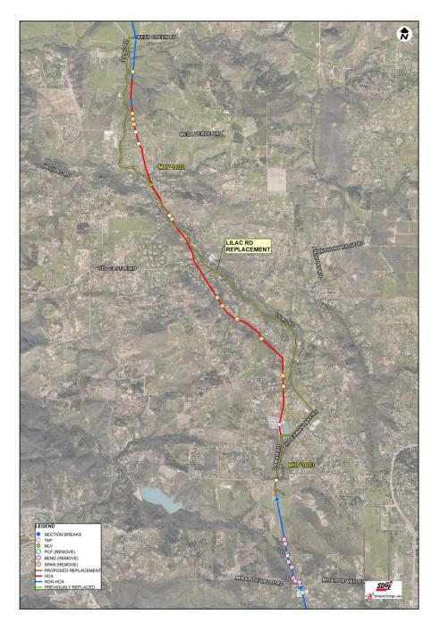
Figure 13 Replace in HCA/Test in Non-HCA Detail Map
