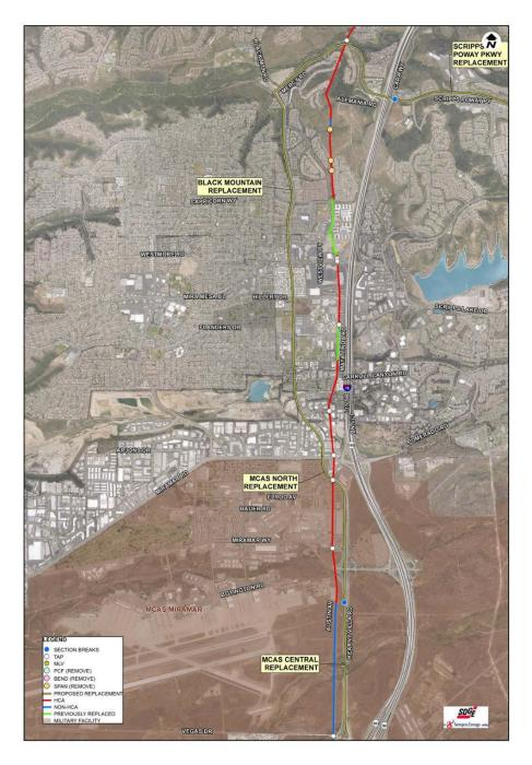
Figure 18 Replace in HCA/Test in Non-HCA Detail Map
