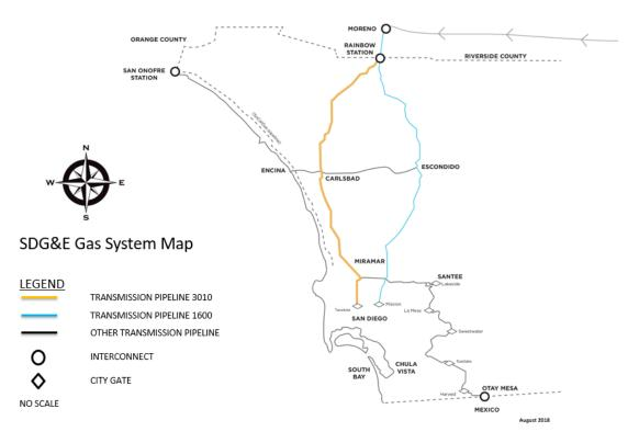
Figure 2: SDG&E Gas Transmission System
