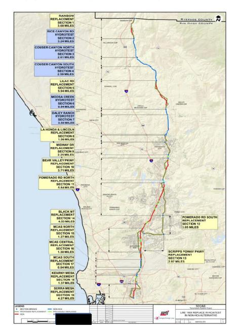
Figure 1: Map of Plan to Primarily Replace in HCAs, Hydrotest in Non-HCAs<sup>7</sup>
