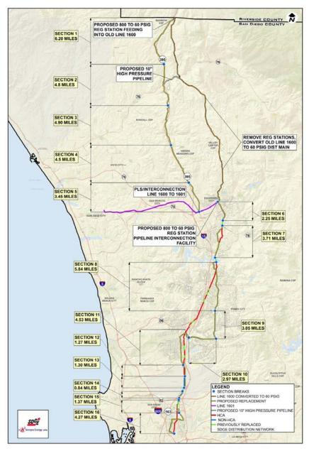
Figure 8: Full Replacement Along Highway 395 Alternative
