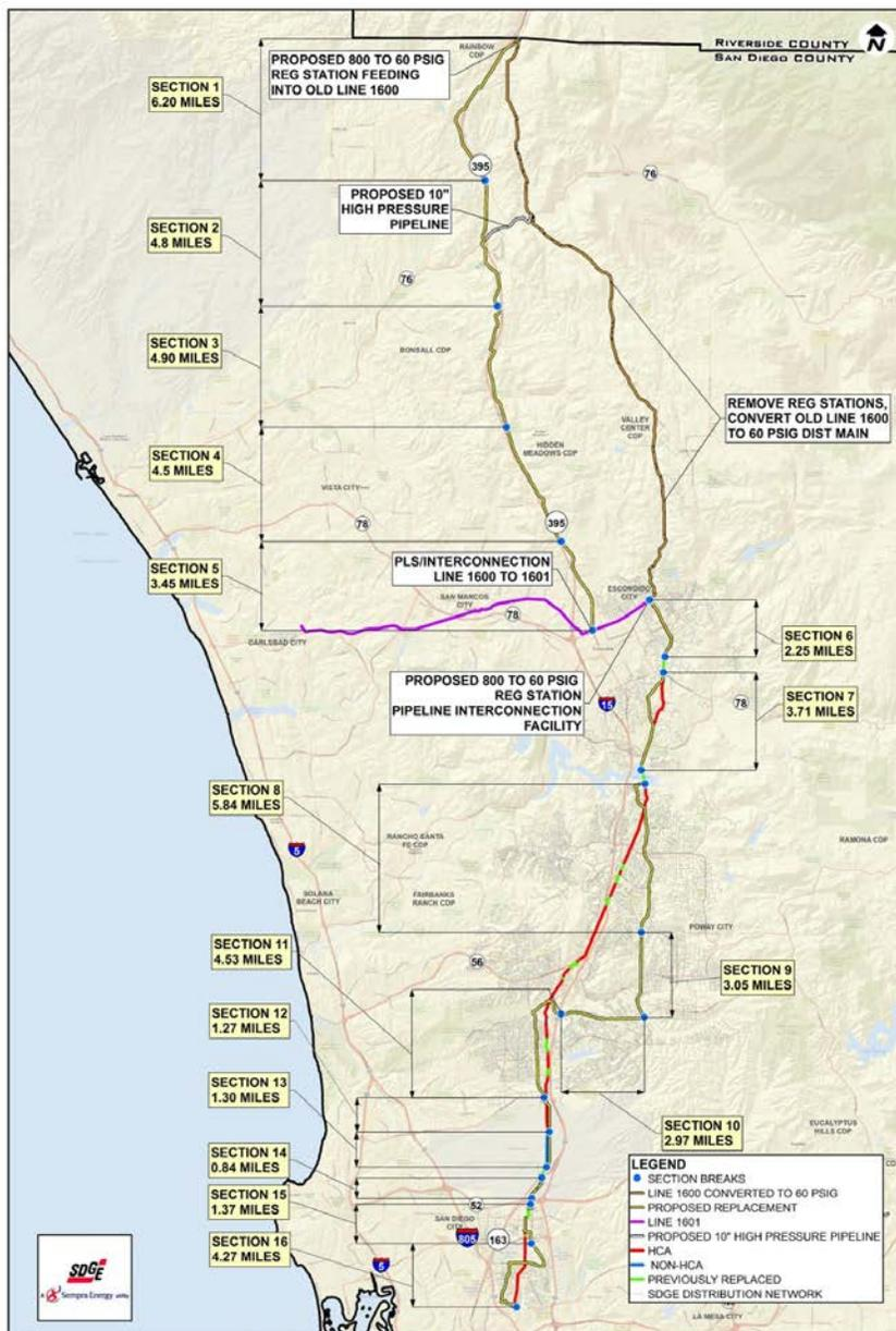
Figure 9: Preliminary Schedule Full Replacement Along Highway 395 Alternative
