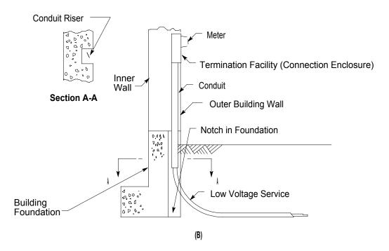
(Alternate to (A) for Recessed Connection Enclosure)
