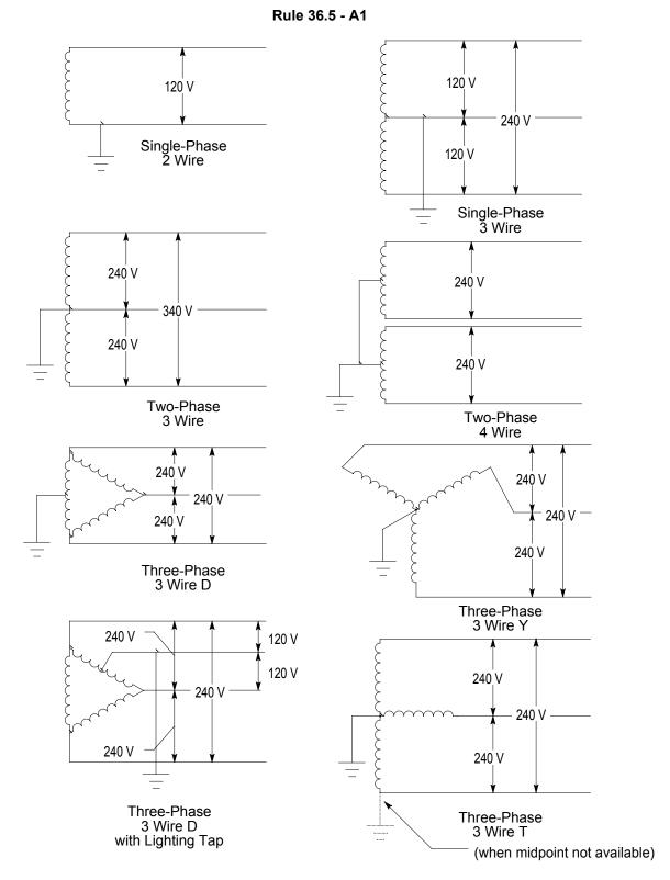
**Figure 16**Grounding of Transformer Windings
