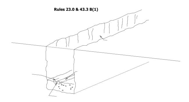
**Figure 5**Random Separation of Buried Cable
