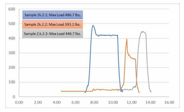
Figure 6-17: Slip Load Test – 35kV, 1/0 AWG ACSR with
