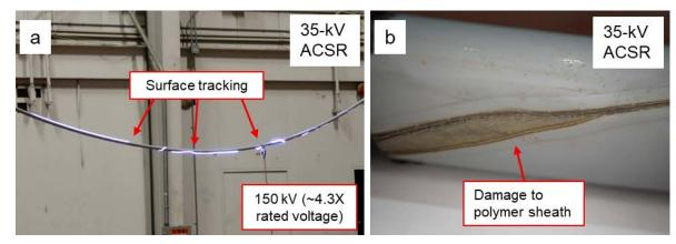
Figure 18. (a) Surface tracking during breakdown test at 150 kV in the 35-kV ACSR CC. (b) Damage to the surface of the CC due to sustained exposure to high-voltage corona and surface tracking.
