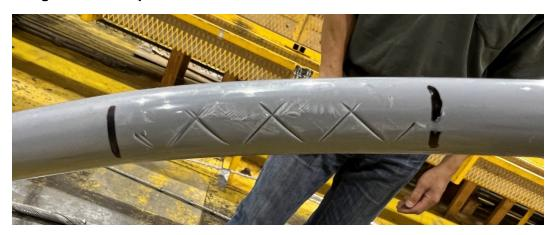
Figure 6-8: Sample 3.1.1 - 17 kV, 1/0 AWG ACSR Condition after Test
