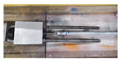
Figure 6-10: Sample 1.2.3 after test (failed at epoxy dead-end)
