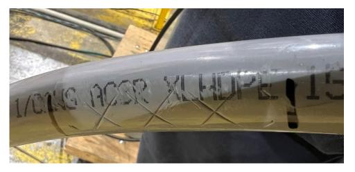
Figure 6-15: Sample 3.2.2 - 35 kV, 1/0 AWG ACSR Condition after Test
