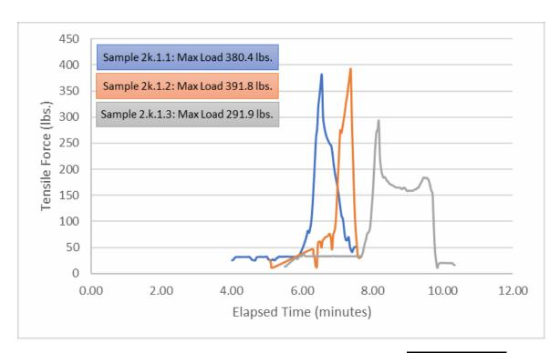
Figure 6-16: Slip Load Test – 17kV, 1/0 AWG ACSR with
