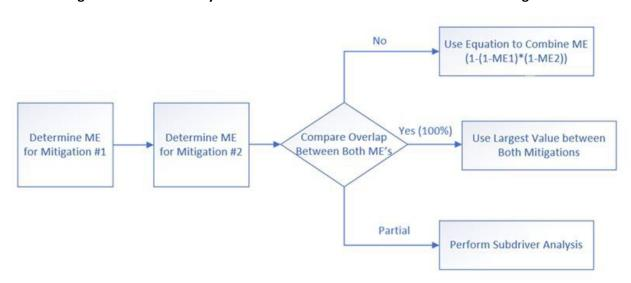
Figure 8 SCE Preliminary Framework – Calculation of a Combination of Mitigations
