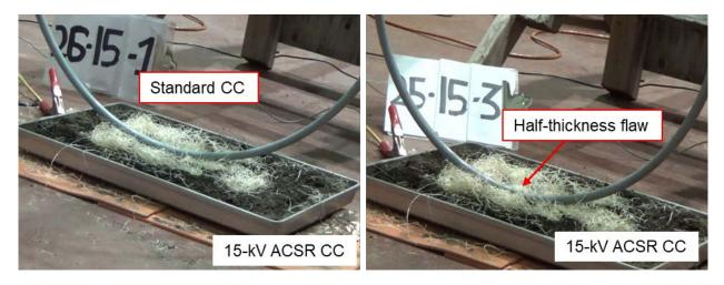
Figure B5. (Left) Simulated wire-down test of a 15-kV ACSR CC. No ignition was observed after three tests. (Right) Simulated wire-down test of a 15-kV ACSR CC with a half-thickness flaw. No ignition was observed after three tests.
