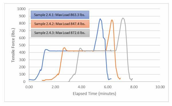
Figure 6-15: Slip Load Test – 15kV, 1/0 AWG ACSR with
