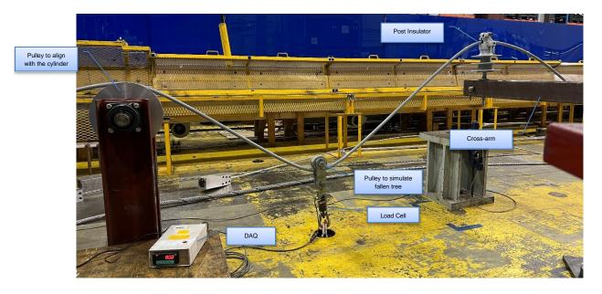
Figure 4-2: Full Mock-up Test - Picture of the Setup
