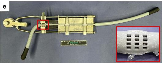
Figure 26. Representative images showing (a) Ripley and (b) manual stripping techniques and (c) creviced end (intended to mimic poor workmanship), (d) midspan artificial damage (to simulate abrasion), and (e) IPCs (inset shows pierced CC area after IPC is removed) used throughout testing.
