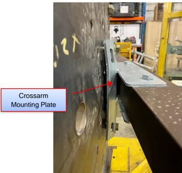
Figure 6-13: Sample 2.3 - Failure Location
