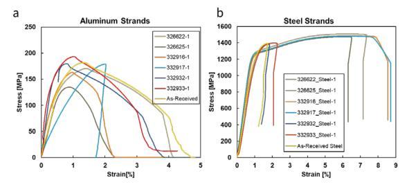
Figure 44. Engineering stress-strain curves for salt-spray-tested (a) aluminum and (b) steel strands from covered and bare 15-kV ACSR conductors. Sample IDs starting with 326622 and 332625 are from salt-spray-tested CCs with IPC hardware. Sample IDs starting with 332916 and 332917 are from salt-spray-tested CCs with midspan damage. Sample IDs starting with 332932 and 332933 are from a salt-spray-tested bare conductor. The as-received sample is also a bare conductor.
