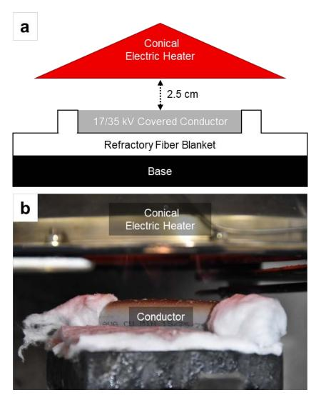
Figure 54. (a) Schematic and (b) representative photo of the heat flux testing apparatus. The top edge of the CC was spaced 2.5 cm from the bottom of the conical heat source. A refractory fiber blanket was used to provide an adiabatic back surface and protect the ends of the CC to reduce unwanted edge effects.
