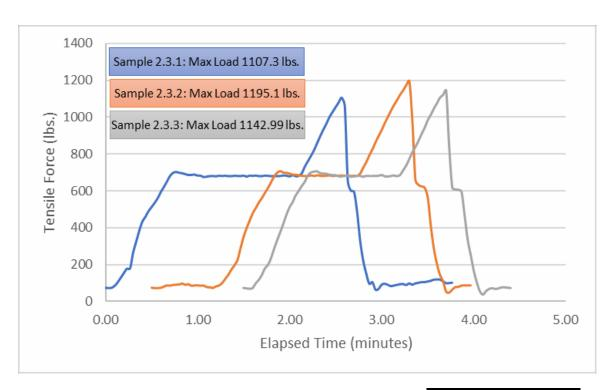
Figure 6-14: Slip Load Test – 22kV, 397.5 kcmil AAC with
