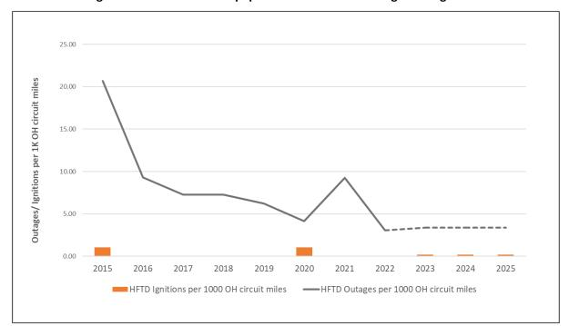
Figure 8-5: Transmission Equipment related HFTD Outages and Ignitions
