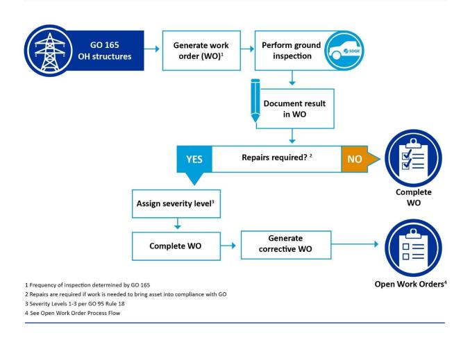
Distribution patrol inspections are currently completed on an annual basis on all structures, including those in the HFTD. Non-routine patrol inspections may occur for safety, reliability, or operational needs. For example, patrol inspections are performed on all distribution structures potentially affected by or affected by a PSPS event prior to and after the PSPS event.
