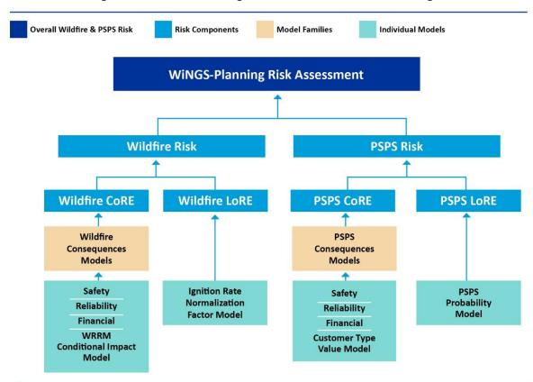
Figure 6-4: WiNGS-Planning Risk Calculation Process Flow Diagram
