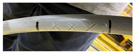
Figure 6-10: Sample 3.1.2 - 17 kV, 1/0 AWG ACSR Condition after Test
