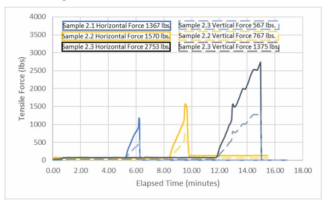
Figure 6-2: Test Load Profile: 17kV 2/0 AWG, 19 CU Conductor
