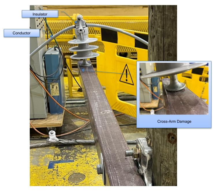
Figure 6-21: Sample 3.4.1 – Insulator and Cross-arm Condition after Test
