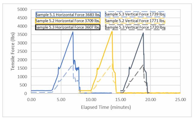
Figure 6-5: Test Load Profile: 17kV 336.4 KCMIL, 18/1 ACSR Conductor
