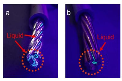
Figure 31. Representative photographs of (a) 17-kV ACSR and (b) 17-kV copper conductors after water ingress testing and sheath removal. Fluorescence was observed between the individual strands as well as around the core.
