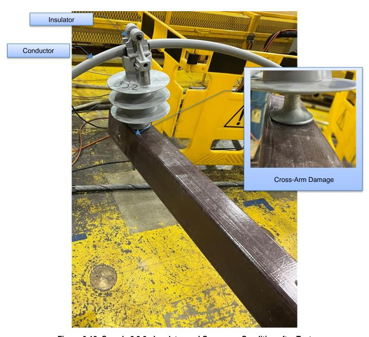
Figure 6-18: Sample 3.3.2 - Insulator and Cross-arm Condition after Test
