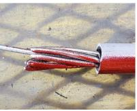
Figure 6-6: Sample 1.1.2 after test (conductor failed at South end of splice)
