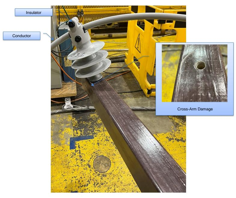
Figure 6-17: Sample 3.3.1 – Insulator and Cross-arm Condition after Test
