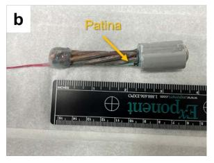
Figure 49. Representative pre-test photographs of aged (a) 17-kV ACSR and (b) 17-kV copper CCs. The immersion aging resulted in patina formation on copper conductors.
