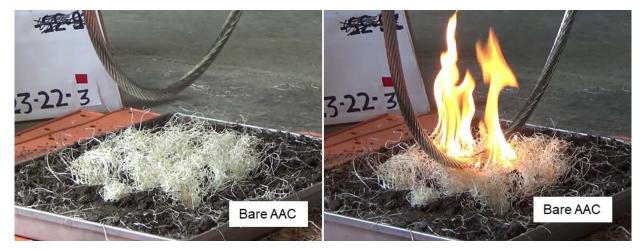
Figure B2. Simulated wire-down test of a bare AAC demonstrating the potential for ignition of the dry brush.
