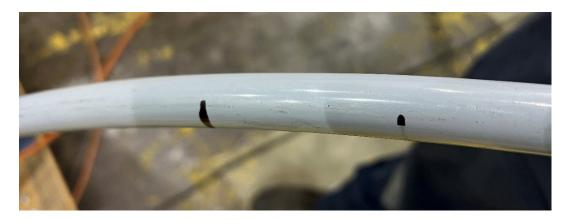
Figure 6-34: Sample 3K.1.3 - 17 kV, 1/0 AWG ACSR Condition after Test
