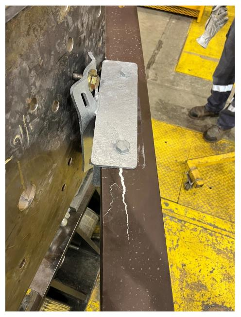
Figure 6-17: Sample 4.1 - Failure Location
