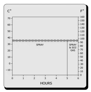
Figure 34.  $SO_2$ /salt fog test conditions. The chamber was held at 35° C  $\pm$  2° C and salt fog was introduced continually for 168 hours.  $SO_2$  was introduced for one hour out of every six, as indicated. From ASTM G85-19: Standard Practice for Modified Salt Spray (Fog) Testing.<sup>22</sup>
