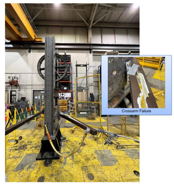
Figure 6-22: Sample 6.1 – Failure Location
