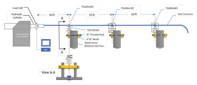
Figure 60. Schematic diagram of insulator slip test.
