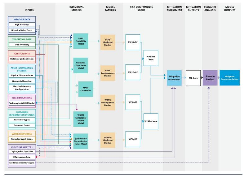
Figure 6-7: WiNGS-Planning Calculation Schematic
