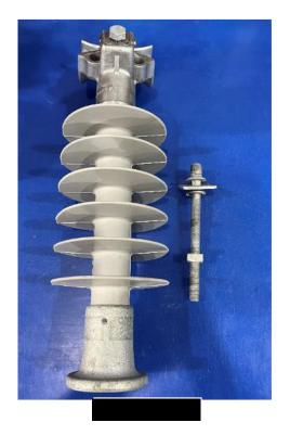
Figure 6-11: - Typical Insulator and Pin Condition after Slip Test (no damage)
