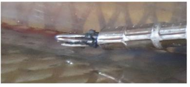
Figure 6-8: Sample 1.2.1 after test (conductor failed at North end of splice)
