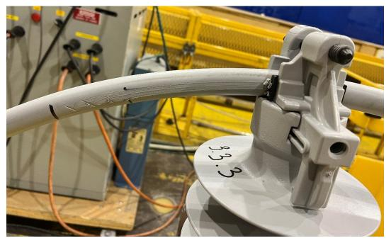
Figure 6-20: Sample 3.3.3 - 22 kV, 397.5 kcmil AAC Condition after Test
