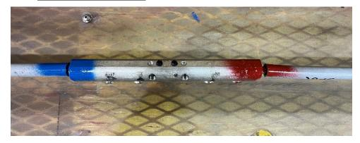
Figure 3-5: Installed on 15 kV 1/0 AWG, 6/1 ACSR
