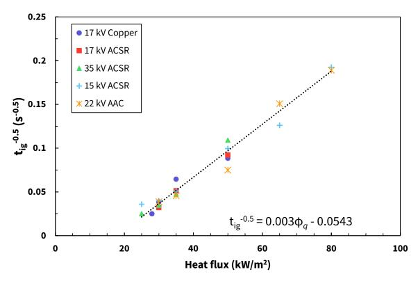
Figure 55. Symbols portray the autoignition time (plotted as the inverse square root) as a function of incident heat flux from cone calorimetry tests. The line is a linear best fit providing a correlation between heat flux and ignition times for the CCs.
