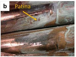
Figure 53. Representative optical microscopy images of (a) stripped and (b) covered portions of an unaged cyclic polarization tested 17-kV copper CC.
