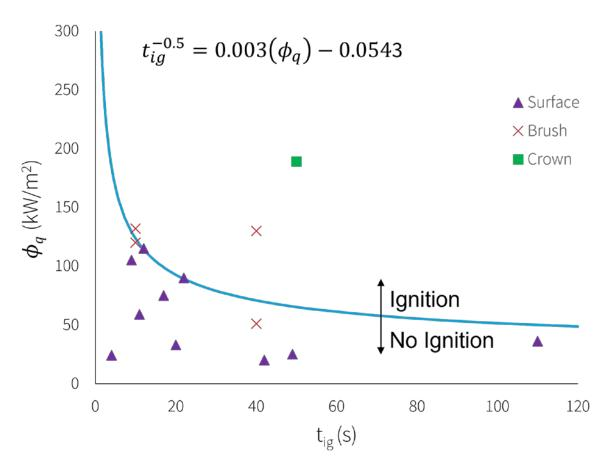
Figure 56. Critical heat flux and associated residence time for autoignition. Symbols represent full-scale wildland fire data. The blue line represents the theoretical minimum heat flux required for autoignition derived from cone calorimetry experiments and thermally thick ignition theory.
