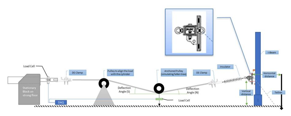
Figure E1. Schematic diagram of the dead-end tree fall test. The hydraulic actuator is located on the south end (left), and the cross-arm is located on the north end (right).
