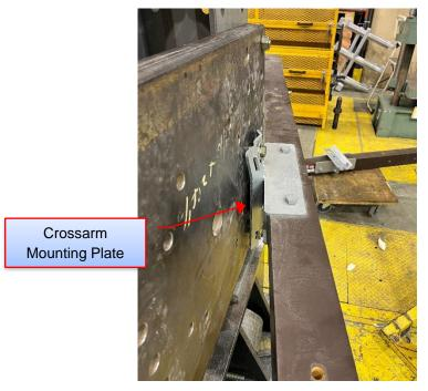
Figure 6-16: Sample 3.3 - Failure Location
