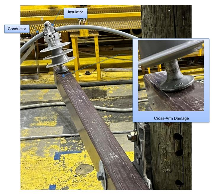
Figure 6-13: Sample 3.2.1 – Insulator and Cross-arm Condition after Test
