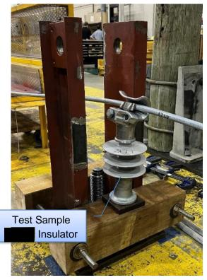
Figure 4-2: Clamp Slip Test Setup
