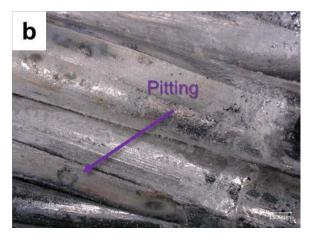
Figure 51. Representative optical microscopy images of (a) stripped and (b) covered portions of an unaged cyclic-polarization-tested 17-kV ACSR CC.
