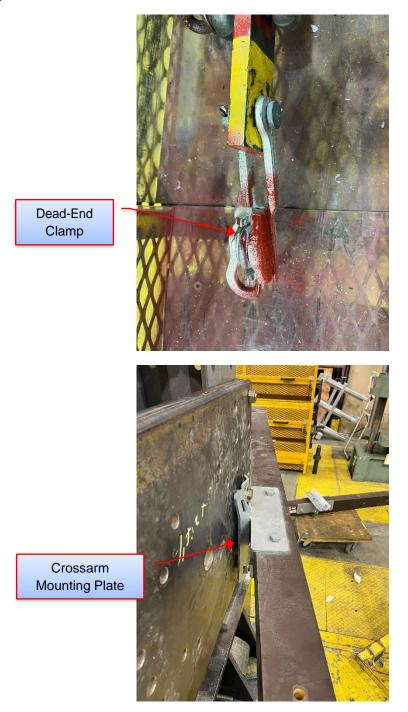
Figure 6-15: Sample 3.2 - Failure Location
