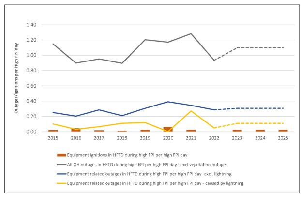
Figure 8-3: Distribution Equipment related HFTD Ignitions and Outages Rate
