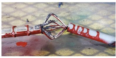
Figure 6-7: Sample 1.1.3 after test (conductor failed at North epoxy dead-end)
