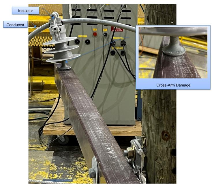
Figure 6-16: Sample 3.2.3 – Insulator and Cross-arm Condition after Test
