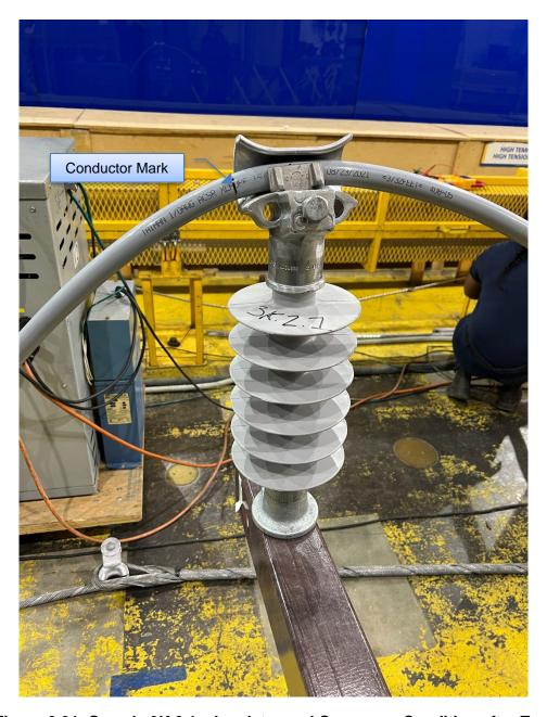
Figure 6-31: Sample 3K.2.1 – Insulator and Cross-arm Condition after Test
