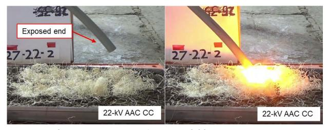
Figure B4. Simulated wire-down test of a 22-kV AAC CC with a broken end demonstrating the potential for ignition of the dry brush.
