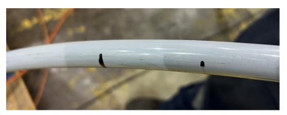
Figure 6-30: Sample 3K.1.3 - 17 kV, 1/0 AWG ACSR Condition after Test
