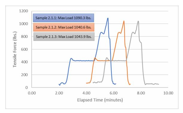
Figure 6-12: Slip Load Test – 17kV, 1/0 AWG ACSR with
