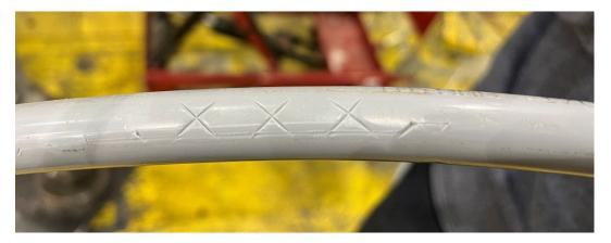
Figure 6-24: Sample 3.4.3 - 15 kV, 1/0 AWG ACSR Condition after Test
