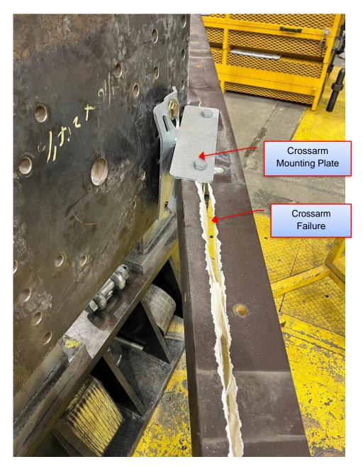
Figure 6-27: Sample 7.3 - Failure Location
