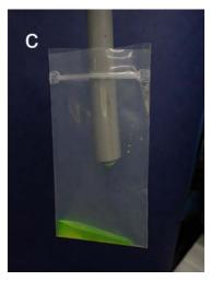
Representative photographs of liquid ingress testing performed on 17-kV ACSR CCs. (a) Liquid was introduced to the stripped end of a 17-kV ACSR CC at t=0. (b-c) After five minutes, the liquid level had dropped significantly at the stripped end (b), and liquid output was observed at the far end of the CC (c).
