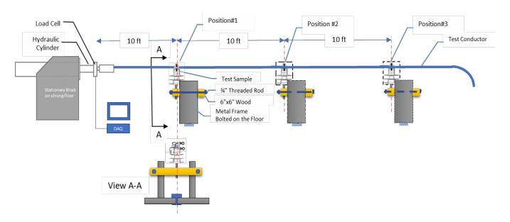
Figure 4-1: Clamp Slip Test Schematic
