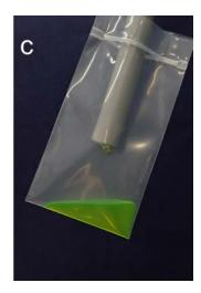
Figure 29. Representative photographs of liquid ingress testing performed on 17-kV copper CCs. (a) Liquid was introduced to the stripped end of a 17-kV copper CC at t=0. (b-c) After five minutes (t=5), the liquid level had dropped significantly at the stripped end (b), and liquid output was observed at the far end of the CC (c).
