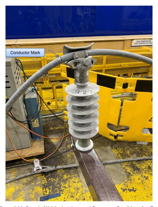
Figure 6-32: Sample 3K.2.2 – Insulator and Cross-arm Condition after Test
