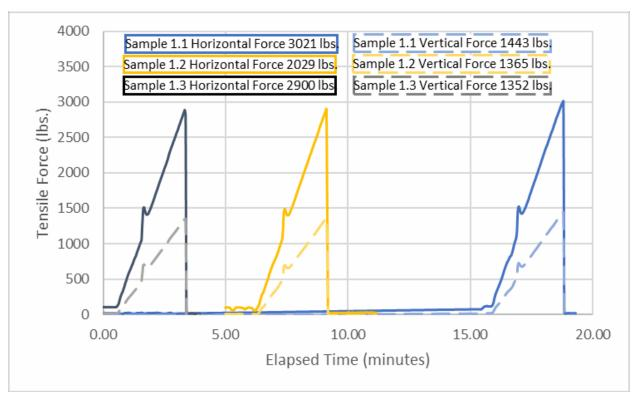
Figure 6-1: Test Load Profile: 17KV #2 AWG, 7 CU Conductor
