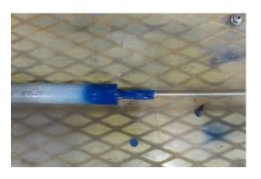
Figure 6-9: Sample 1.2.2 after test (conductor failed at North end of splice)
