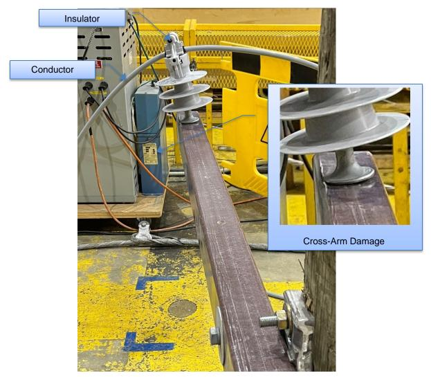
Figure 6-23: Sample 3.4.3 – Insulator and Cross-arm Condition after Test
