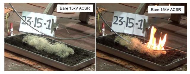
Figure B6. Simulated wire-down test of a bare 15-kV ACSR conductor demonstrating the potential for ignition of the dry brush.
