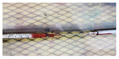
Figure 6-5: Sample 1.1.1 after test (conductor failed at South end of splice)
