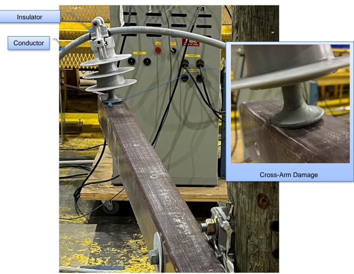
Figure 6-14: Sample 3.2.2 – Insulator and Cross-arm Condition after Test
