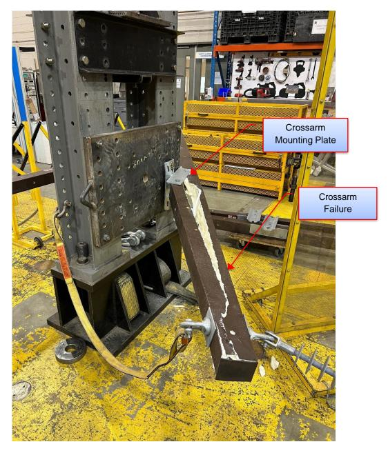
Figure 6-21: Sample 5.3 - Failure Location
