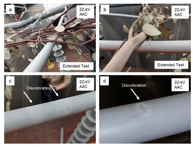
Figure 10. (a,b) Test setup for one-week extended test at rated voltage (22-kV AAC pictured). (c,d) Discoloration on the surface of 22-kV AAC after one week.
