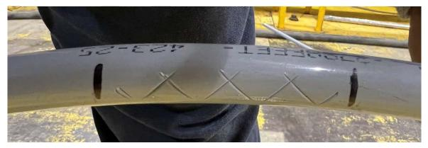
Figure 69. A representative post-test image showing superficial marks on the conductor at the vise-top insulator grip location (17-kV 1/0 ACSR).
