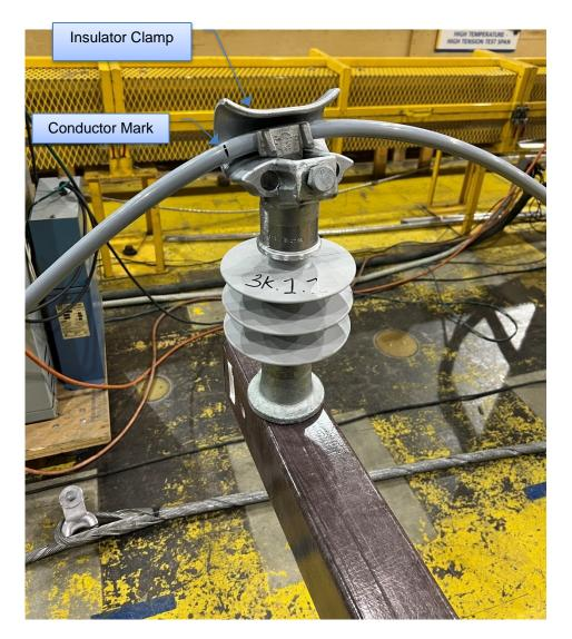
Figure 6-27: Sample 3K.1.2 – Insulator and Cross-arm Condition after Test
