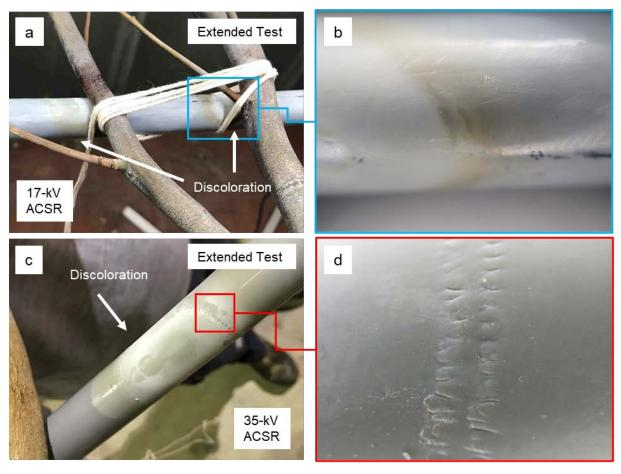
Results of one-week extended contact test at rated voltages. (a) Discoloration on the surface of 17-kV ACSR CC after one week and (b) higher-magnification image of the indicated area in (a). (c) Discoloration and damage on the surface of a 35-kV ACSR after one week, and (d) higher-magnification image of the indicated area in (c).
