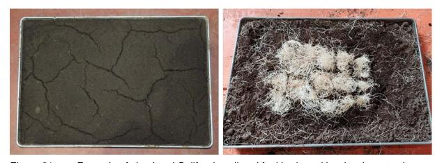
Figure 21. Example of simulated California soil and fuel bed used in wire-down testing.
