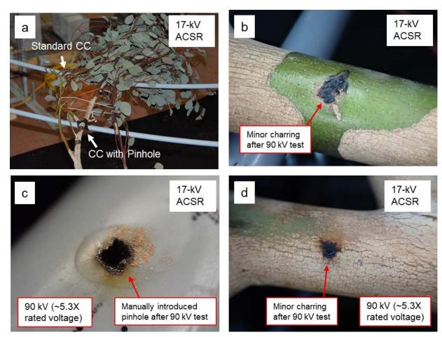
Figure 19. (a) Sequential phase-to-phase contact testing after induced breakdown. (b) Contact point showing minor charring on leafy eucalyptus branch after exposure to 90 kV. (c) Manually introduced pinhole flaw in 35-kV ACSR CC after contact testing at 90 kV. (d) Contact point showing minor charring on leafy eucalyptus branch after exposure to 90 kV.
