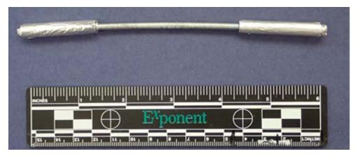
Figure 42. Representative photograph of a tensile specimen with aluminum foil wrapped ends. The aluminum foil reduces the likelihood of failure outside the gauge length.
