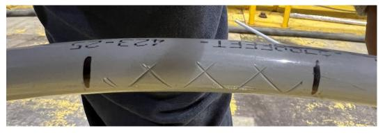
Figure 6-12: Sample 3.1.3 - 17 kV, 1/0 AWG ACSR Condition after Test
