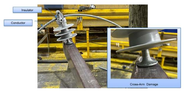
Figure 70. A representative post-test image showing insulator deformation and damage to the cross-arm at its connection point (35-kV 1/0 ACSR).
