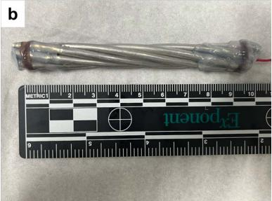
Figure A10. Representative photographs showing (a) CC and (b) bare conductor samples prepared for cyclic polarization testing. Electrical contact was made to one end of the conductor with conductive silver epoxy. The electrical connection and the other exposed end of the conductor were masked with silicone sealant.
