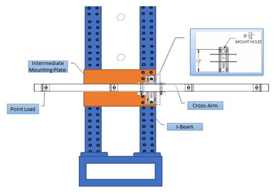
Figure 4-2: Full Mock-up: Front View of the Setup
