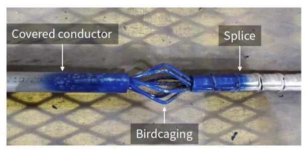
Figure 65. A representative photograph showing the birdcaging behavior of splices on 17-kV and 35-kV ACSR CCs.
