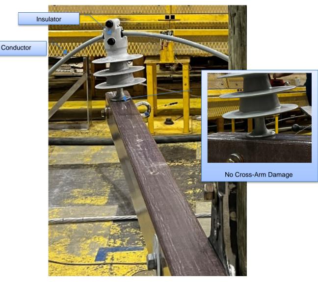
Figure 6-9: Sample 3.1.2 - - Insulator and Cross-arm Condition after Test
