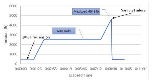
Figure 59. Representative load vs. time plot for the splice maximum load test (Test 1.1).
