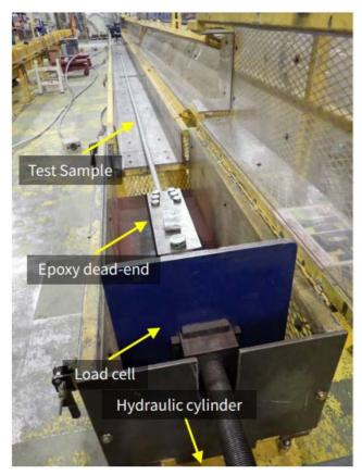
Figure 58. Representative photo of splice maximum load test.
