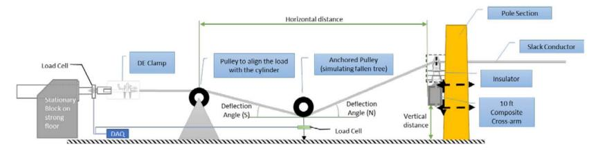
Figure 63. Schematic diagram of the full-system tree-fall test.
