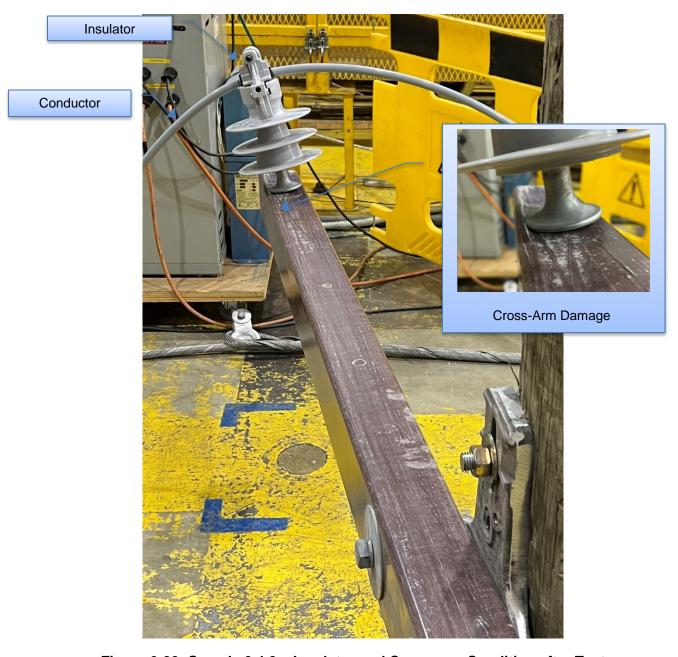
Figure 6-22: Sample 3.4.2 – Insulator and Cross-arm Condition after Test
