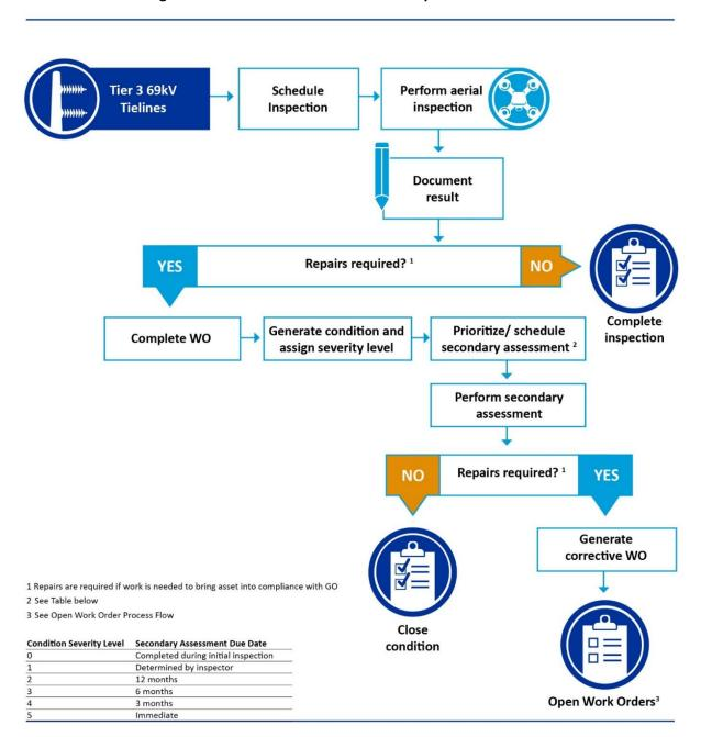
Figure 8-16: Transmission Tier 3 69 kV Inspections Process Flow
