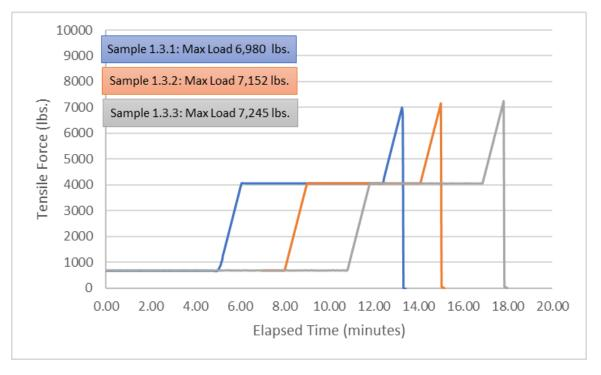
Figure 6-3: Maximum Load Test – 22 kV, 397.5 kcmil AAC
