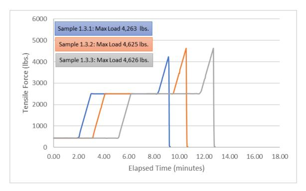
Figure 6-4: Maximum Load Test – 15 kV, 1/0 AWG ACSR
