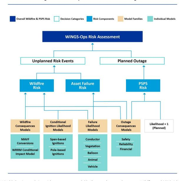
Figure 6-5: WiNGS-Ops Calculation Process Flow Diagram
