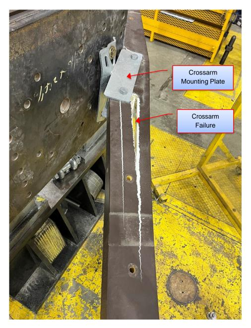
Figure 6-26: Sample 7.2 - Failure Location
