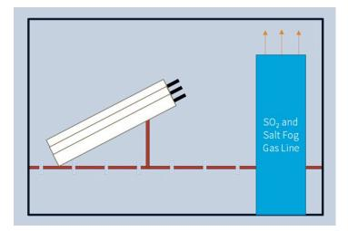
Figure 33. Schematic of salt spray testing apparatus. SO<sub>2</sub> and 5 wt.% salt fog were introduced through a central tube. Samples were arranged on a plastic platform with grid openings to prevent pooling of runoff. The samples were oriented approximately 60–75° from vertical.
