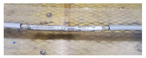
Figure 3-4: Installed on 22 kV 397.5 kcmil, 19 strands AAC
