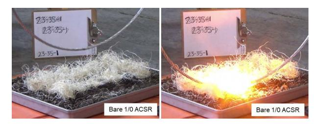
Figure 23. Simulated wire-down test of a bare ACSR conductor demonstrating the potential for ignition of the dry brush.
