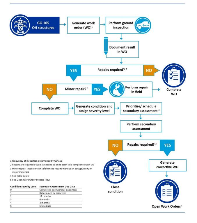
Detailed inspections are currently completed on a 3-year cycle for all overhead structures, including those in the HFTD. Inspections are prioritized and scheduled based on safety, reliability, and operational need.
