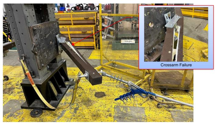
Figure 6-23: Sample 6.2 - Failure Location
