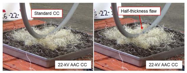
Figure B1. (Left) Simulated wire-down test of a 22-kV AAC CC. No ignition was observed after three tests. (Right) Simulated wire-down test of a 22-kV AAC CC with a half-thickness flaw. No ignition was observed after three tests.
