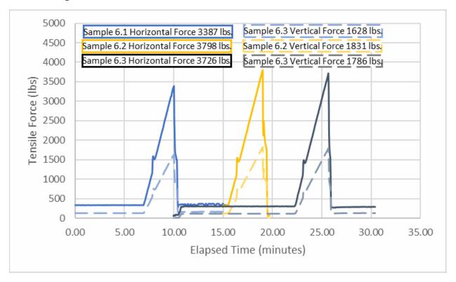
Figure 6-6: Test Load Profile: 17kV 336.4 KCMIL, 30/7 ACSR Conductor
