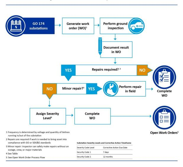
Figure 8-17: Substation Patrol Inspection Workflow
