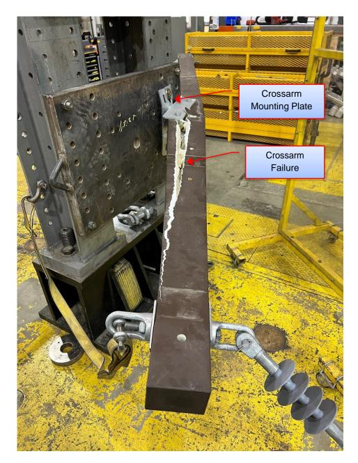
Figure 6-25: Sample 7.1 – Failure Location
