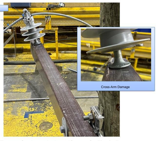
Figure 6-11: Sample 3.1.3 – Insulator and Cross-arm Condition after Test
