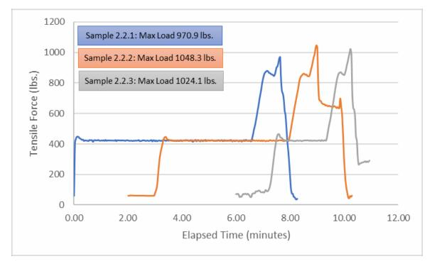
Figure 6-13: Slip Load Test - 35kV, 1/0 AWG ACSR with
