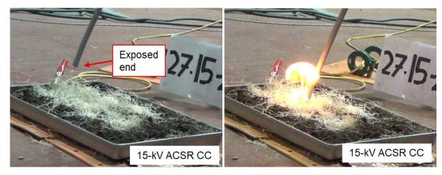
Figure B8. Simulated wire-down test of a 15-kV ACSR CC with a broken end demonstrating the potential for ignition of the dry brush.
