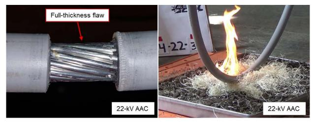
Figure B3. Simulated wire-down test of a 22-kV AAC CC with a full-thickness flaw demonstrating the potential for ignition of the dry brush.
