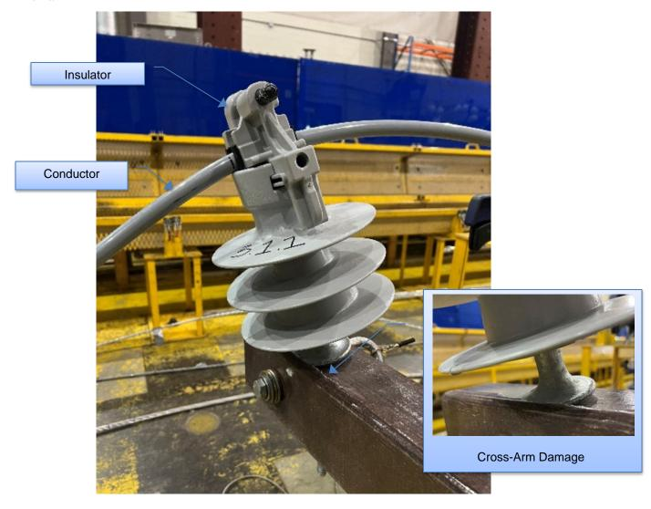
Figure 6-7: Sample 3.1.1 – Insulator and Cross-arm Condition after Test
