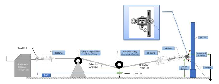
Figure 4-1: Full Mock-up: General View of the Test Setup
