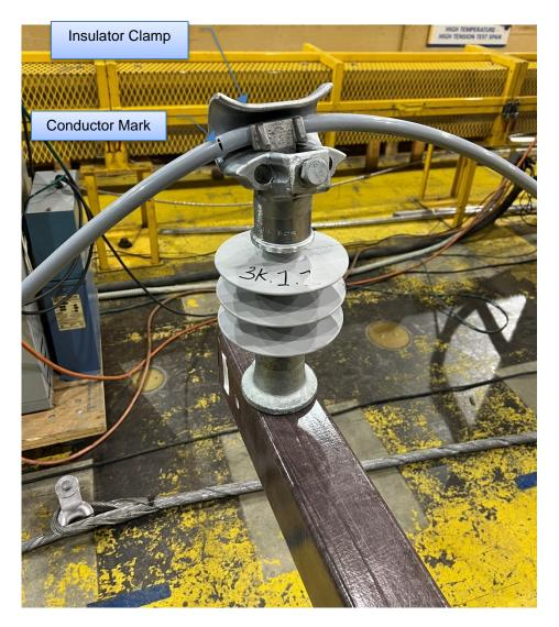
Figure 6-25: Sample 3K.1.1 – Insulator and Cross-arm Condition after Test
