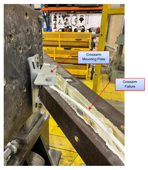
Figure 6-20: Sample 5.1 - Failure Location
