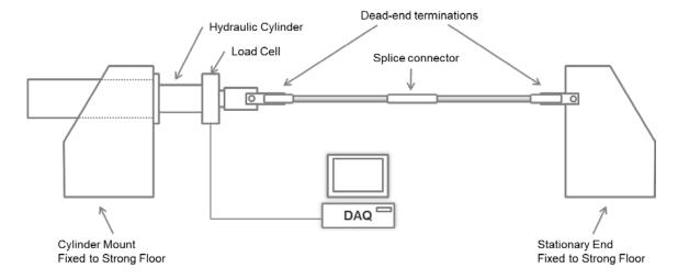
Figure 4-1: Maximum Load Test – Schematic of the Setup
