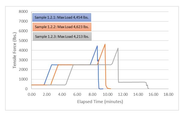
Figure 6-2: Maximum Load Test – 35 kV, 1/0 AWG ACSR
