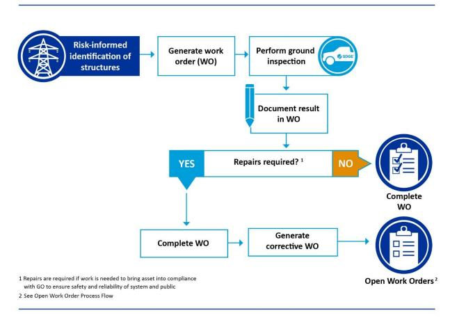
Figure 8-9: Distribution Infrared Inspections Process Flow
