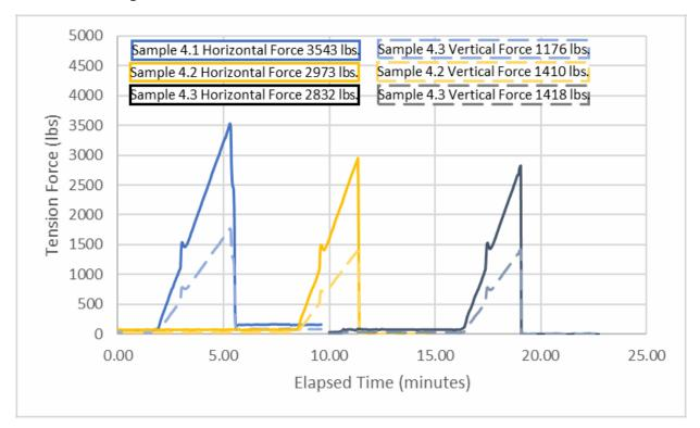
Figure 6-4: Test Load Profile: 17kV 1/0 AWG, 6/1 ACSR Conductor
