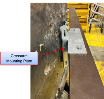
Figure 6-19: Sample 4.3 - Failure Location
