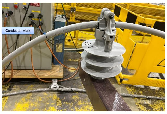
Figure 6-19: Sample 3.3.3 - Insulator and Cross-arm Condition after Test
