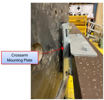
Figure 6-18: Sample 4.2 - Failure Location
