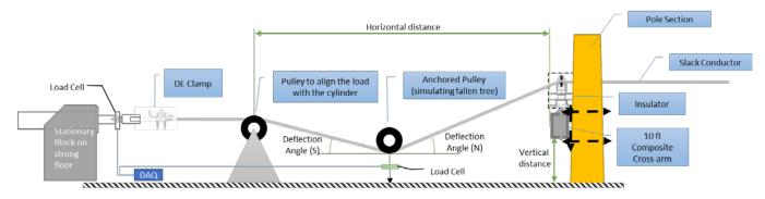
Figure 4-1: Full Mock-up Test - Schematic of the Setup
