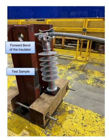
Figure 6-9: - Typical Clamp and 1/0 AWG ACSR (35 kV) Conductor Position after Slip Test
