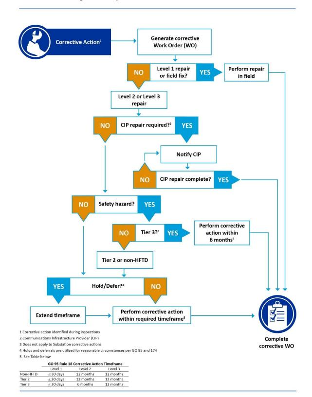
Figure 8-22: Open Work Orders: Corrective Maintenance
