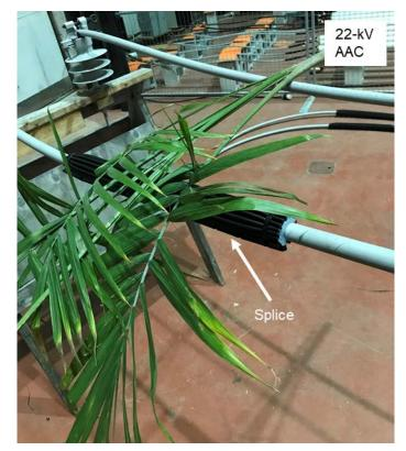
Figure 5. Rated voltage testing of a spliced CC and a standard CC bridged by a palm frond (22-kV AAC pictured).
