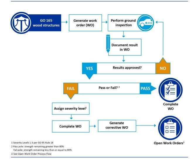
Distribution Wood Pole Intrusive inspections are currently performed on a 10-year cycle. Non-routine intrusive inspections may occur when current pole strength (percent strength remaining) information is needed for pole loading calculations during design work per GO 95.
