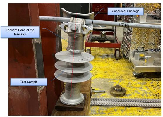
Figure 6-7: - Typical Clamp and 1/0 AWG ACSR (17 kV) Conductor Position after Slip Test
