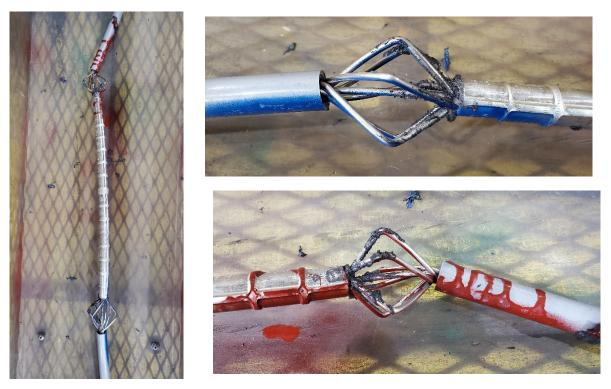
Figure 6-7: Sample 1.1.3 after test (conductor failed at North epoxy dead-end)
