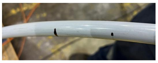
Figure 6-34: Sample 3K.1.3 - 17 kV, 1/0 AWG ACSR Condition after Test
