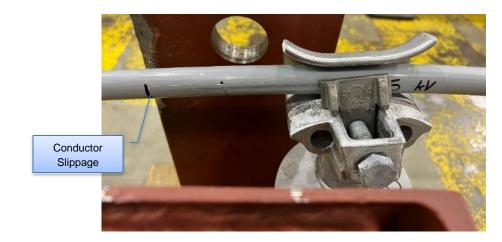
Figure 6-10: - Typical 1/0 AWG ACSR (35 kV) Conductor Condition after Slip Test
