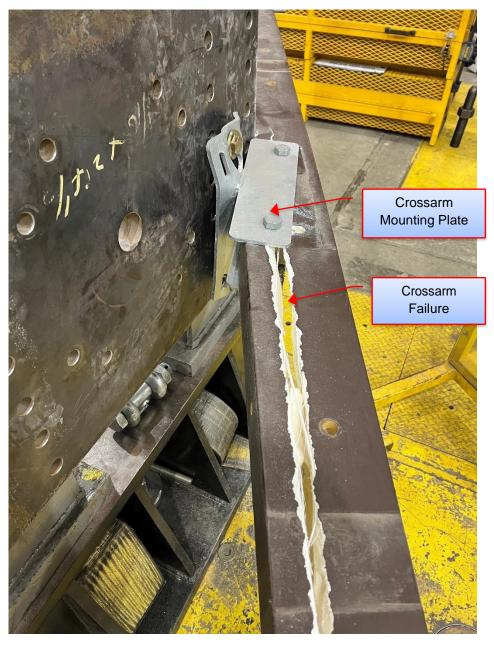
Figure 6-27: Sample 7.3 – Failure Location
