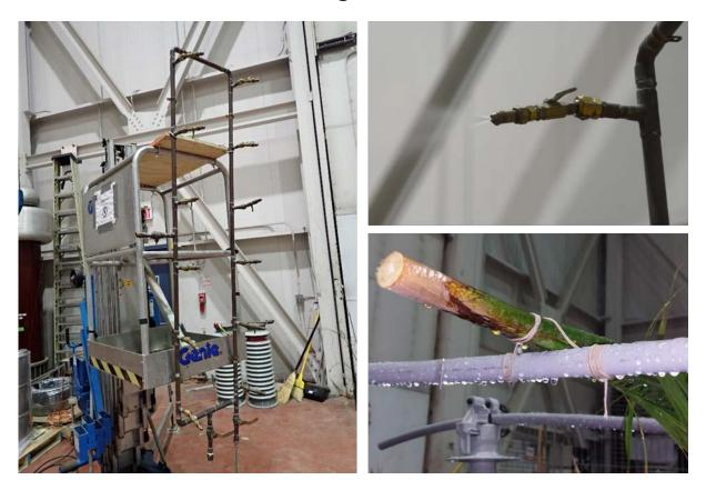
Figure A4. Wet test setup for phase-to-phase contact tests.
