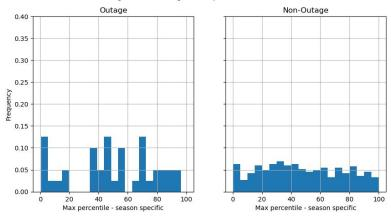
Outage v/s non-outage wind speed max %ile - spring
