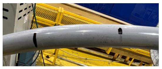
Figure 6-26: Sample 3K.1.1 - 17 kV, 1/0 AWG ACSR Condition after Test
