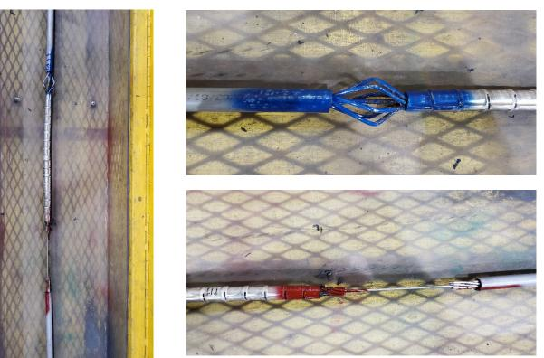
Figure 6-5: Sample 1.1.1 after test (conductor failed at South end of splice)
