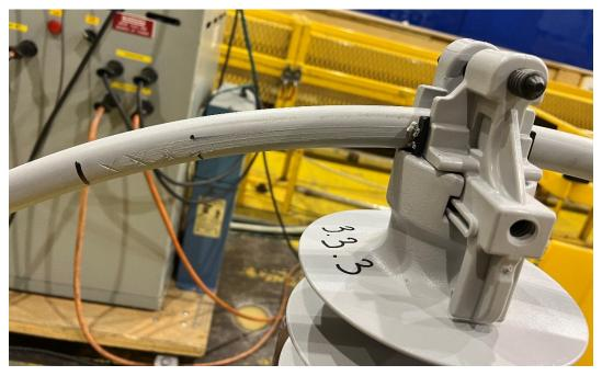
Figure 6-20: Sample 3.3.3 - 22 kV, 397.5 kcmil AAC Condition after Test
