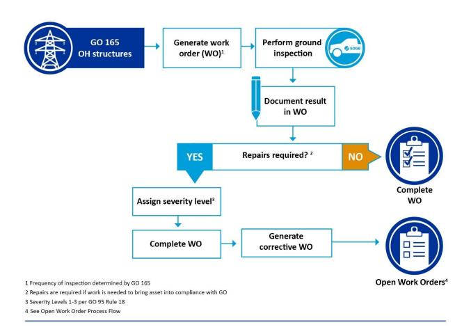
Distribution patrol inspections are currently completed on an annual basis on all structures, including those in the HFTD. Non-routine patrol inspections may occur for safety, reliability, or operational needs. For example, patrol inspections are performed on all distribution structures potentially affected by or affected by a PSPS event prior to and after the PSPS event.
