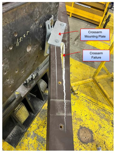
Figure 6-26: Sample 7.2 – Failure Location
