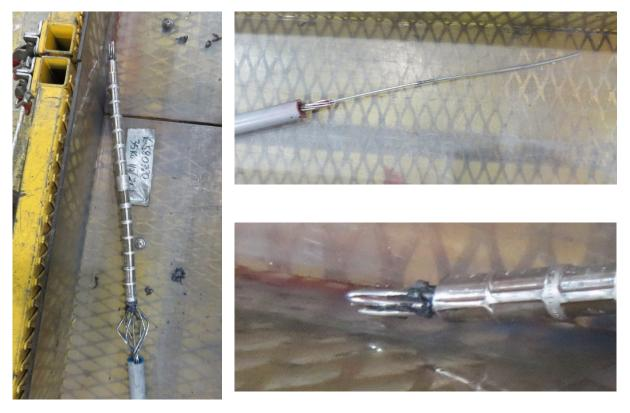
Figure 6-8: Sample 1.2.1 after test (conductor failed at North end of splice)
