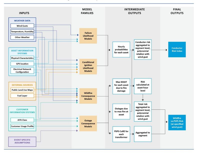
Figure 6-8: WiNGS-Ops Calculation Schematic
