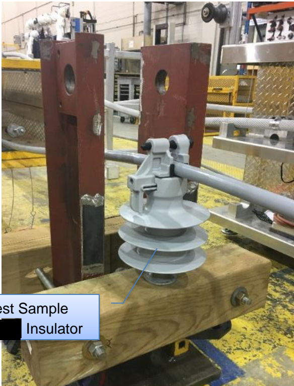
Figure 4-2: Clamp Slip Test Setup
