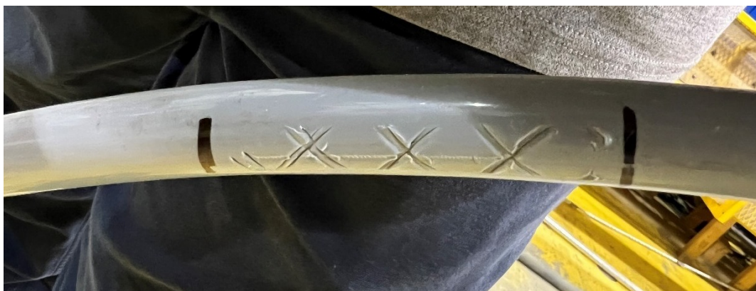
Figure 6-10: Sample 3.1.2 - 17 kV, 1/0 AWG ACSR Condition after Test
