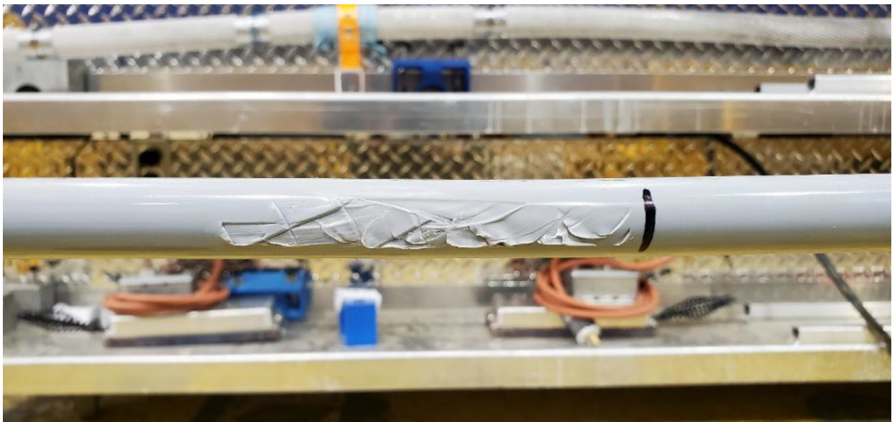
Figure 6-2: [REDACTED] - Typical 1/0 AWG (17 kV) ACSR Conductor Condition after Slip Test
