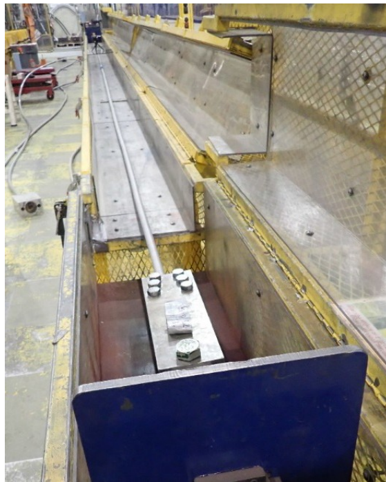
Figure 4-2: Maximum Load Test - Typical Setup
