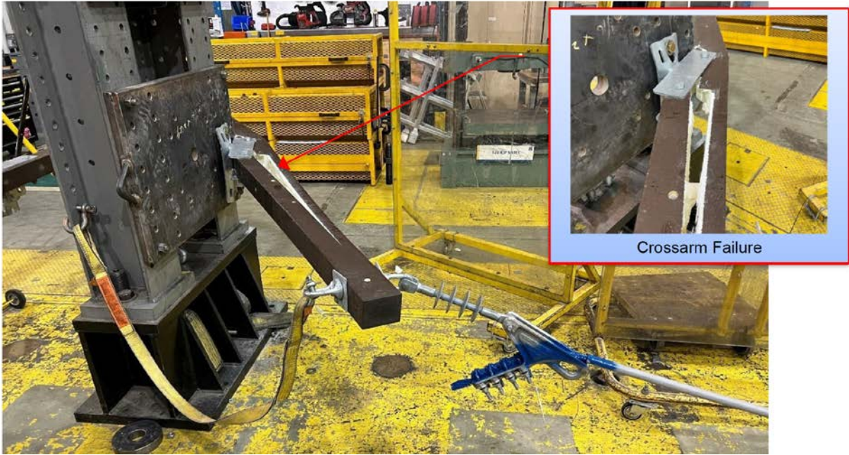
Figure E4. A representative post-test image showing splitting and failure of the composite cross-arm. 336.4 kcmil ACSR (30/7) with Type C dead-end shown.
