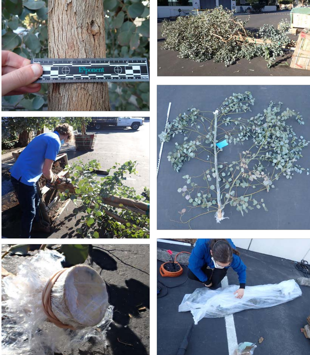
Figure A5. Cutting and preparation of leafy eucalyptus branches for phase-to-phase arc testing.
