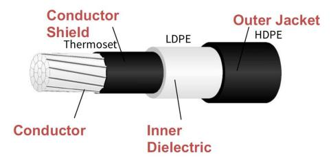
Figure 1. A schematic illustration of a three-layer CC. Diagram modified from Hendrix Aerial Cable Systems [Trager].
