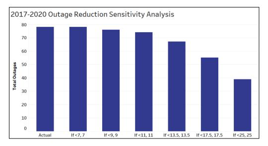
This shows that when trees are brought up to non-enhanced levels (7-11) there is smaller impact to outage reduction. When tree line clearances are brought to above 12 (13.5+), there starts to be a significant impact to potential outage reduction.
