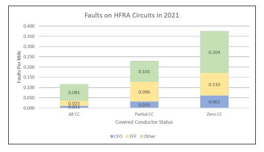
Figure 8: SCE Faults on HFRA Circuits in 2021
