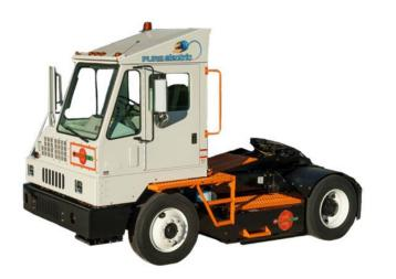
Weight Class (GVWR): Class 8 (33,001+ lbs) **Payload:** 81,000 lbs Chassis/Body Type: Yard Tractor Energy Storage Capacity: 80, 160 kWh **Range:** 50, 100 miles Max Charge Rate: 80 kW **Availability:** Production **Base Price:** \$200,000-\$280,000 Website: https://orangeev.com
