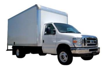
Weight Class (GVWR): Class 4 (14,001-16,000 lb) Payload: 5,088 lbs Chassis/Body Type: Cutaway Energy Storage Capacity: 108, 144 kWh Range: 100-125 miles Max Charge Rate: Not available **Availability:** Pre-production **Base Price:** \$211,000 Website: https://www.alphamobility.co/
