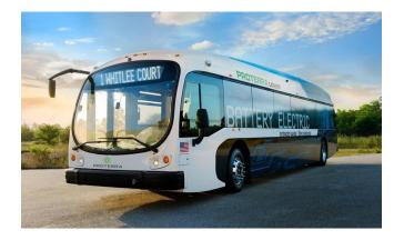
Sales Contact: Bill Williams Director, Commercial Sales bwilliams@proterra.com Weight Class (GVWR): Class 8 (33,001+ lbs) Passenger Capacity: 29 and 40 people **Chassis/Body Type:** Transit Bus Energy Storage Capacity: 225 kWh Range: 91-125 miles Max Charge Rate: 133 kW (plug in); 177 kW (overhead) Availability: In production Base Price: \$609,000 Website: https://www.proterra.com/
