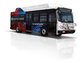
Sales Contact: Patrick Duan Vice President of Operations patrick.duan@byd.com Weight Class (GVWR): Class 8 (33,001+ lbs) Passenger Capacity: 48-56 people **Chassis/Body Type:** Transit Bus Energy Storage Capacity: 352 kWh, 446 kWh, 578 kWh Range: 198 miles Max Charge Rate: 150 kW Availability: In production **Base Price:** Customized Website: <u>http://en.byd.com/usa/</u>
