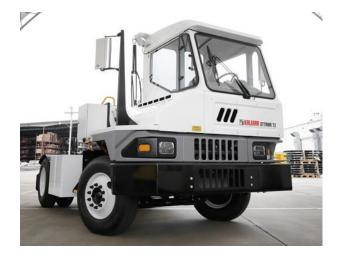
Sales Contact: Donald Lawerence Sales Manager Terminal Tractors <u>dlawrence@papemh.com</u> Weight Class (GVWR): Class 8 (33,001+ lbs) **Payload:** 78,200 Chassis/Body Type: Yard Tractor Energy Storage Capacity: 132-200 kWh Range: 8-20 hrs Max Charge Rate: 70 kW Availability: In production **Base Price:** \$272,000-\$349,000 Website: https://kalmarottawa.com/
