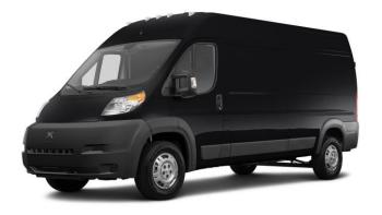
Weight Class (GVWR): Class 2 (6,001-10,000 lbs) **Payload:** 4,100 lbs (4,600 lbs tow) Chassis/Body Type: Van Energy Storage Capacity: 54-75 kWh **Range:** 100-200 miles Max Charge Rate: 200 kW Availability: In production **Base Price:** \$34,990 - \$45,000 Website: https://www.maxwellvehicles.com/
