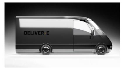
Weight Class (GVWR): Class 3 (10,001-14,000 lb) Payload: Not available Chassis/Body Type: Van Energy Storage Capacity: 70, 105, 140, 175, 210 kWh Range: 200 miles Max Charge Rate: 100 kW **Availability:** Pre-production **Base Price:** \$125,000 Website: https://bollingermotors.com/bollinger-b2/
