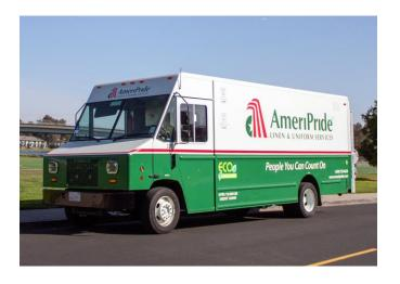
Sales Contact: John Felts Sales Representative NorCal & NW USA john.felts@motivps.com Weight Class (GVWR): Class 6 (19,501-26,000 lbs) **Payload:** 10,000 lbs **Chassis/Body Type:** Stripped Chassis Energy Storage Capacity: 127 kWh Range: 105 miles Max Charge Rate: 60 kW **Availability:** In production **Base Price:** Customized; available upon request Website: <a href="https://www.motivps.com/motivps/">https://www.motivps.com/motivps/</a> portfolio-items/epicf59-allelectric-stepvan/
