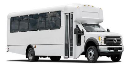
Sales Contact: Julie Johnson Enterprise Business Development julie.johnson@lightningsystems.com Weight Class (GVWR): Class 5 (16,001-19,500 lbs) Passenger Capacity: Not available Chassis/Body Type: Shuttle Bus Energy Storage Capacity: 128 kWh Range: 110 miles Max Charge Rate: 80 kW
