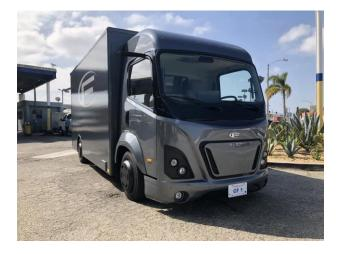
Weight Class (GVWR): Class 3 (10,001-14,000 lb) **Payload:** 4,800 lbs **Chassis/Body Type:** Straight/Box Truck Energy Storage Capacity: Not available Range: 100 miles Max Charge Rate: Not available **Availability:** Pre-production **Base Price:** Not available Website: <a href="https://www.cityfreighter.com/">https://www.cityfreighter.com/</a>
