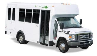
Weight Class (GVWR): Class 4 (14,001-16,000 lbs) Passenger Capacity: 28 people Chassis/Body Type: Shuttle Bus Energy Storage Capacity: 88 kWh Range: 100 miles Max Charge Rate: 13 kW Availability: In production **Base Price:** \$283,000 Website: https://mbcbus.com/product/d-series/
