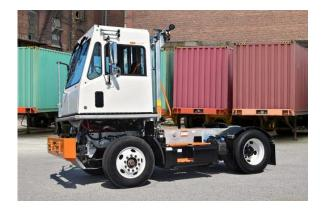
Weight Class (GVWR): Class 8 (33,001+ lbs) **Payload:** 42,000 Chassis/Body Type: Yard Tractor Energy Storage Capacity: 132, 172, 196 kW Range: Not available Max Charge Rate: Not available Availability: Pre-production **Base Price:** \$275,000–\$310,000
