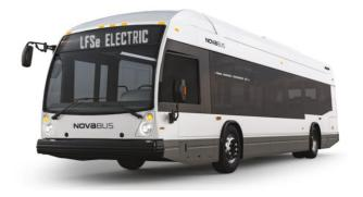
Sales Contact: Denton Shuey denton.shuey@volvo.com Weight Class (GVWR): Class 7 (26,001-33,000 lbs) Passenger Capacity: 68-71 poeple **Chassis/Body Type:** Transit Bus Energy Storage Capacity: 564 kWh **Range:** 211-292 miles Max Charge Rate: 150 kW (depot), 450 kW (on-route) Availability: In production **Base Price:** Not available Website: http://novabus.com/
