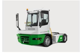
Sales Contact: Ron Van Arkel R.vanArkel@terbergamericas.com Weight Class (GVWR): Class 8 (33,001+ lbs) Payload: 130,000 Chassis/Body Type: Yard Tractor Energy Storage Capacity: 96, 148, 222 kW Range: 5.5, 8, 12 hours Max Charge Rate: 96 kW
