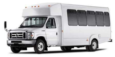
Sales Contact: Julie Johnson Enterprise Business Development julie.johnson@lightningsystems.com Weight Class (GVWR): Class 4 (14,001-16,000 lbs) **Passenger Capacity:** 24 people Chassis/Body Type: Shuttle Bus Energy Storage Capacity: 86 kWh,129 kWh Range: 80-120 miles Max Charge Rate: 80 kW **Availability:** In production **Base Price:** Customized
