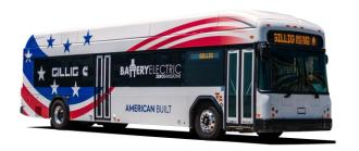
Sales Contact: Bus Sales (510) 785-1500 sales@gillig.com Weight Class (GVWR): Class 8 (33,001+ lbs) Passenger Capacity: 35 people **Chassis/Body Type:** Transit Bus Energy Storage Capacity: 296 kWh, 444 kWh Range: Not available Max Charge Rate: Not available Availability: In production **Base Price:** Not available Website: <a href="https://www.gillig.com/">https://www.gillig.com/</a>
