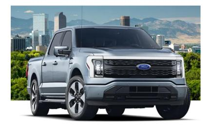
Weight Class (GVWR): Class 2 (6,001-10,000 lbs) Payload: 2,000 lbs Chassis/Body Type: Pickup **Energy Storage Capacity:** Not available **Range:** 230-300 miles Max Charge Rate: 19.2 kW Availability: In production **Base Price:** \$39,974 Website: <u>https://www.ford.com/...</u>
