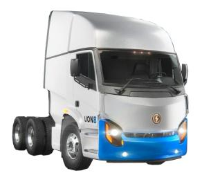
Sales Contact: Dave Anderson Sales Manager <u>dave.anderson@thelionelectric.com</u> Weight Class (GVWR): Class 8 (33,001+ lbs) **Payload:** 30,000 lbs Chassis/Body Type: Tractor Energy Storage Capacity: 588 kWh Range: 210 miles Max Charge Rate: 100 kW Availability: In production **Base Price:** \$300,000 Website: https://thelionelectric.com/en
