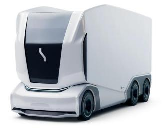
Weight Class (GVWR): Class 8 (33,001+ lbs) **Payload:** 35,000 lbs Chassis/Body Type: Tractor Energy Storage Capacity: 200-300 kWh Range: 80-186 miles Max Charge Rate: Not available Availability: In production **Base Price:** \$10,000 (monthly service fee up to \$22,500) Website: https://www.einride.tech/
