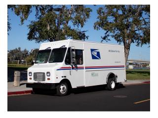
Sales Contact: John Felts Sales Representative NorCal & NW USA john.felts@motivps.com Weight Class (GVWR): Class 4 (14,000-16,000 lbs) Payload: 5,000-6,000 lbs Chassis/Body Type: Cutaway, Stripped Chassis Energy Storage Capacity: 127 kWh Range: 105 miles Max Charge Rate: 60 kW
