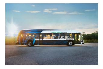
Sales Contact: Bill Williams Director, Commercial Sales bwilliams@proterra.com Weight Class (GVWR): Class 8 (33,001+ lbs) Passenger Capacity: 40 people **Chassis/Body Type:** Transit Bus Energy Storage Capacity: 675 kWh **Range:** 205-329 miles Max Charge Rate: 135 kW (plug in); 407 kW (overhead) Availability: In production **Base Price:** Not available Website: https://www.proterra.com/
