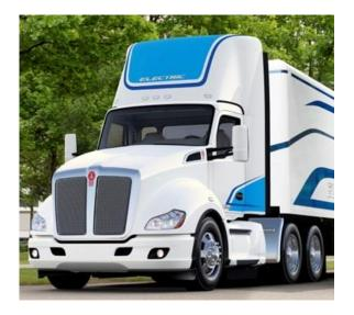
Weight Class (GVWR): Class 8 (33,001+ lbs) Payload: Not available **Chassis/Body Type:** Tractor and straight truck Energy Storage Capacity: 396 kWh **Range:** 100-150 miles Max Charge Rate: 120 kW **Availability:** Production **Base Price:** Not available
