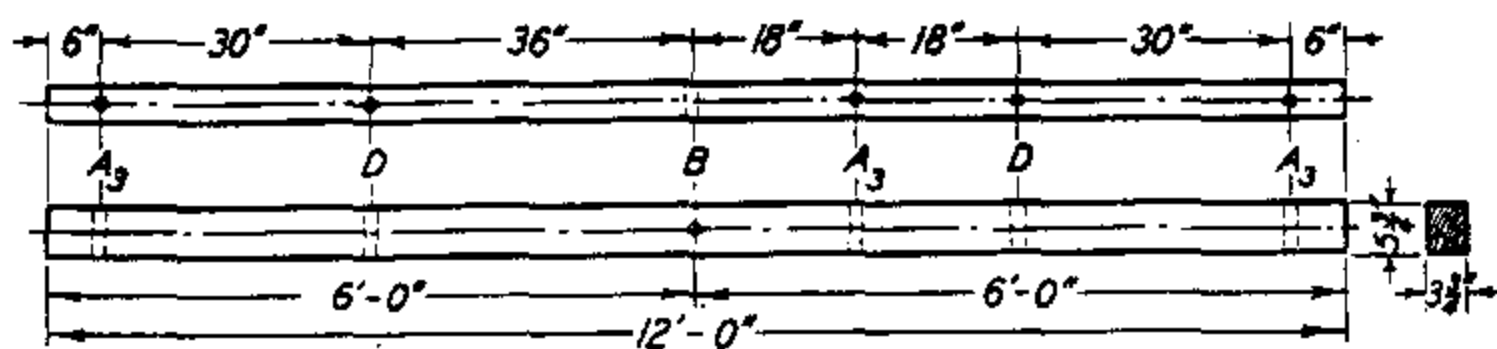
ITEM NO. 1 - LINE POST TANGENT ARM - 0° TO 3° ANGLES (6' BRACE)
