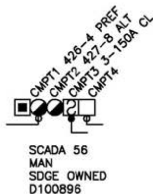
PME SOURCE TRANSFER SCADA
