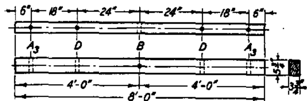
ITEM NO. 4 - LINE POST ARM 69KV ARM FOR TRIANGULAR CONSTRUCTION (4' BRACE)
