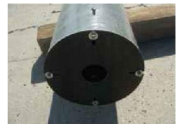
J-BOLTS ON INSIDE OF MODULE
