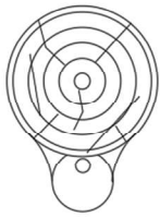
METHOD 1 IMPREGNATED FIBER CONDUIT OF 1/4" MINIMUM THICKNESS
