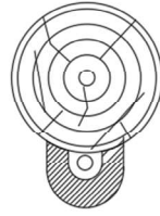
METHOD 2 WOOD MOULDING OF 1 1/2" MINIMUM THICKNESS
