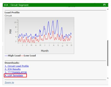
B. In the downloaded LGP Template.csv file, the utility ID (MT\_UTILITY\_NAME), distribution feeder ID (MT\_ASSOCIATED\_FEEDER), three-phase electrical node ID (Node ID), date of the last ICA online refresh date, and precalculated maximum LGP values for each LGP configuration will be prepopulated. The Customer will not alter the .csv file format. The Customer should examine the three pre-populated
