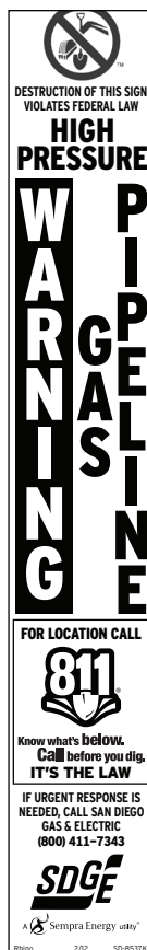
Markers indicate the general location of major pipelines.
