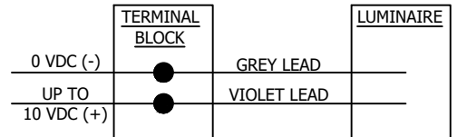
DIAGRAM 2 DIMMING CONTROL SCHEMATIC
