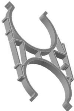
FIGURE 3 5-INCH VERTICAL SPACER FOR 9-INCH WIDTH TRENCH
