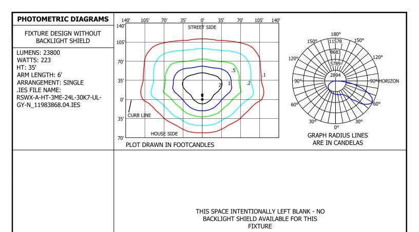
**ATTENTION:** LUMEN OUTPUT "Q" SETTING MUST BE INCLUDED FOR EACH FIXTURE WITHIN THE CONSTRUCTION NOTES FOR EACH LOCATION IN THE JOB PACKAGE.
