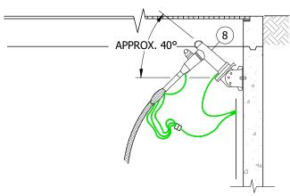
FIGURE 5 3314, 3315 & 3316 HANDHOLES CABLE TAP ANGLE SIDE VIEW
