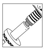
3. PULL OUT THE FUSE HOLDER THREE INCHES AND STOP! WAIT A FEW SECONDS FOR THE OIL TO DRAIN INTO THE TANK. THE INNER FUSE HOLDER ASSEMBLY CAN NOW BE REMOVED WITHOUT DRIPPING EXCESS OIL BY KEEPING THE FUSE HOLDER RUBBING AGAINST THE TOP OF THE CUTOUT, AS SHOWN, AND EXTRACTING IT VERY SLOWLY. THE TOTAL LENGTH OF THE INNER FUSE HOLDER ASSEMBLY, INCLUDING FUSE CARTRIDGE, IS FOURTEEN INCHES.
