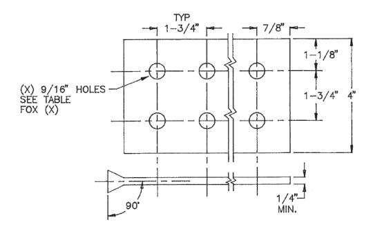
Figure 4 - "T" Spade terminal dimensions.
