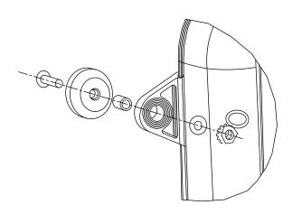
$\frac{\textbf{FIGURE 2}}{\text{MAGNETIC MOUNTING KIT ASSEMBLY (A)}}$
