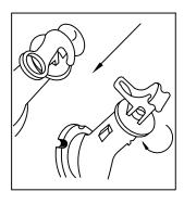
2. PUSH DOWN AND ROTATE THE HANDLE 90° IN THE TUBE. DURING THIS PROCEDURE INTERNAL TANK PRESSURE ESCAPES AND INSIDE AND OUTSIDE PRESSURES ARE EQUALIZED. THE 90° ROTATION OF THE FUSE HOLDER BREAKS ANY ADHESION BETWEEN THE SEAL GASKET AND THE OUTER TUBE ASSEMBLY.
