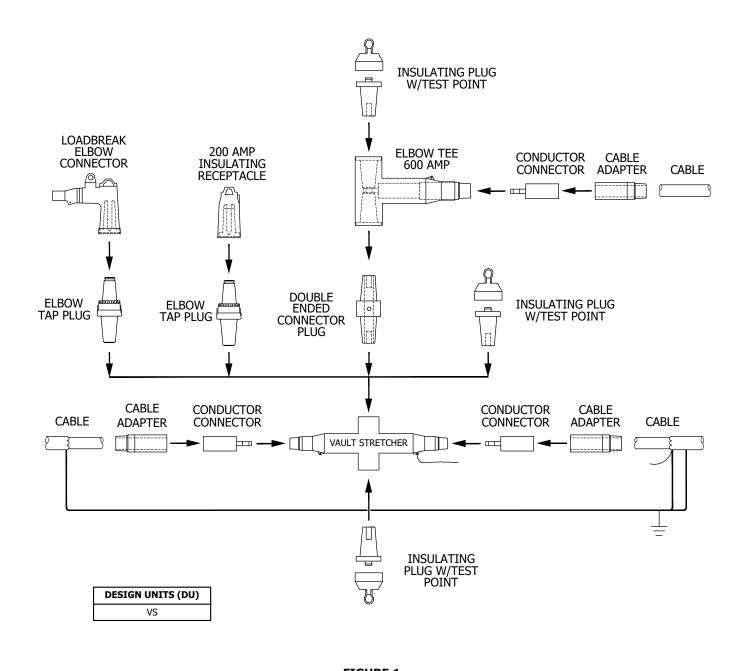
FIGURE 1 VAULT STRETCHER ASSEMBLY (A) [
