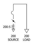
FIGURE 1 IN/OUT WALL MOUNT 200A MANUAL CONNECTION DIAGRAM
