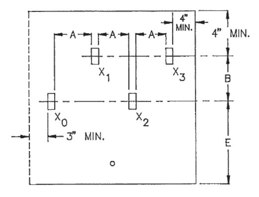
Figure 5 - Secondary bushing spatial diagram.
