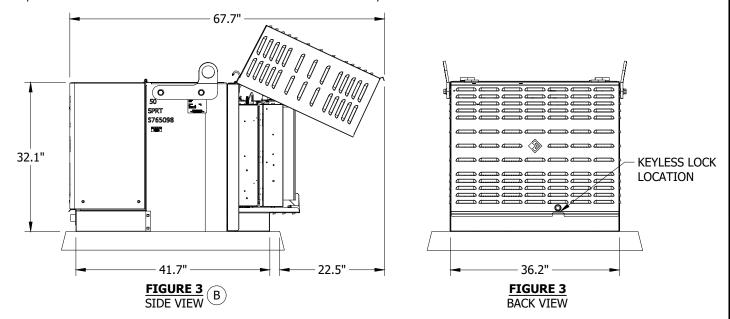
(C) CUSTOM LIFTING BRACKETS HAVE BEEN SUPPLIED DUE TO THE SHIFT OF BALANCE WITH THE ADDITION OF THE INLINE POWER REGULATOR. TURN LIFTING BRACKETS UPSIDE DOWN AFTER INSTALLATION.
