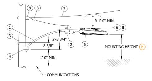
FIGURE 1 6'-0" ARM INSTALLATION
