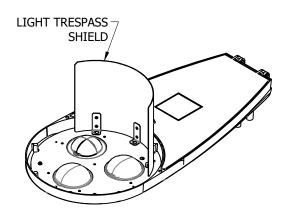
FIGURE 20 ATBM WITH LTS
