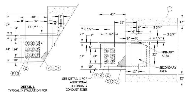
TYPICAL INSTALLATION FOR NINE 3-INCH OR NINE 4-INCH SECONDARY CONDUITS
