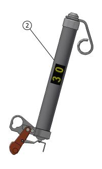
FIGURE 2 SINGLE BARREL ELF FUSE
