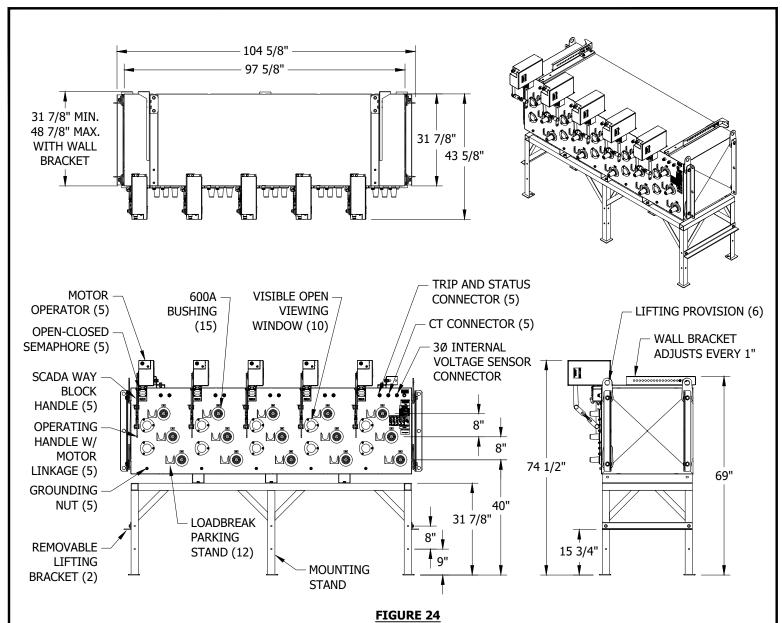
FIVE-WAY VAULT MOUNT 600A SCADA 12KV SEE TABLES 11 AND 12
