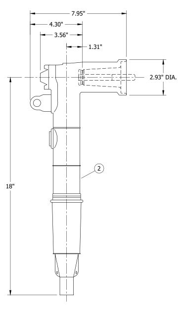
FIGURE 2 200A REPLACEMENT LOADBREAK ELBOW
