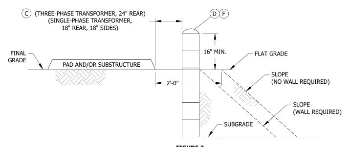
FIGURE 2 MINIMUM CLEARANCE REQUIREMENTS FROM PAD MOUNTED AND/OR SUBSURFACE EQUIPMENT TO REVERSE SUBGRADE RETAINING WALLS
