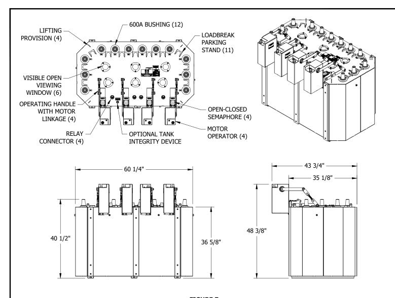
FOUR-WAY SUBMERSIBLE 600A MANUAL/NON-SCADA
