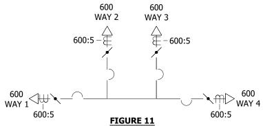
FOUR-WAY SUBMERSIBLE 600A SCADA CONNECTION DIAGRAM
