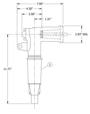
FIGURE 1 200A REPAIR LOADBREAK ELBOW
