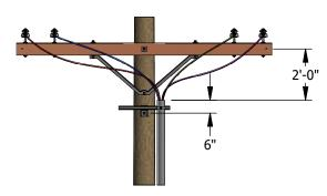
FIGURE 2 OPEN SECONDARY "AIR MAILING" FRONT VIEW
