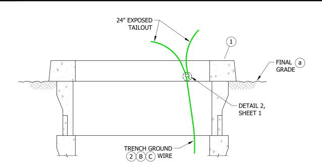
FIGURE 3 PAD WITH 3312 HANDHOLE(S) SECTION VIEW
