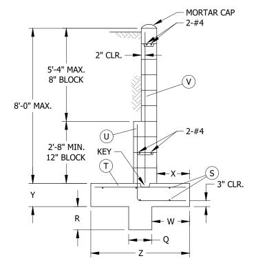
FIGURE 9 C-5 TYPICAL SECTION 5'-4" MAX.
