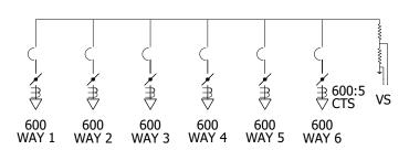
FIGURE 32 SIX-WAY VAULT MOUNT 600A SCADA 12KV CONNECTION DIAGRAM SEE TABLES 15 AND 16
