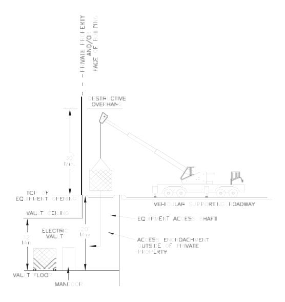
Figure 7 - Access to equipment for Below Grade vaults.
