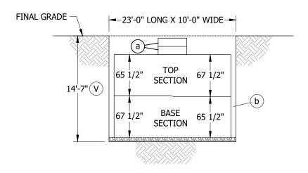
FIGURE 2 **EXCAVATION DIMENSIONS**
