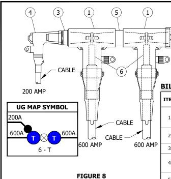
3315 & 3316 HANDHOLE INSTALLATION ONLY SUBSURFACE CONNECTIONS
