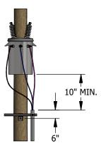
**FIGURE 1** TERMINAL CONSTRUCTION (a) FRONT VIEW
