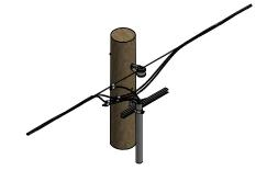
FIGURE 4 SECONDARY AERIAL CABLE TANGENT CONSTRUCTION ISOMETRIC VIEW
