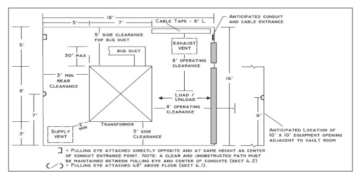
Figure 11 - Typical below grade residential vault configuration for one transformer.
