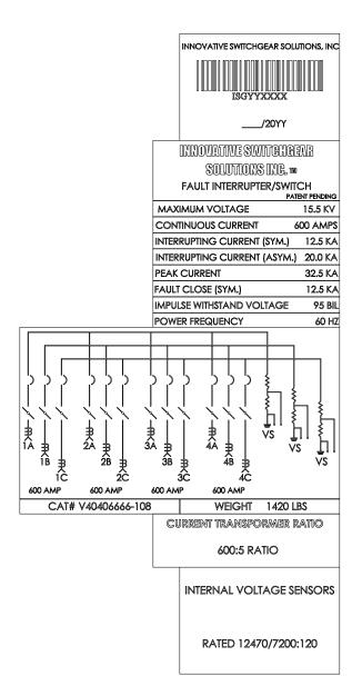
FOUR-WAY VAULT MOUNT 600A MANUAL/NON-SCADA
