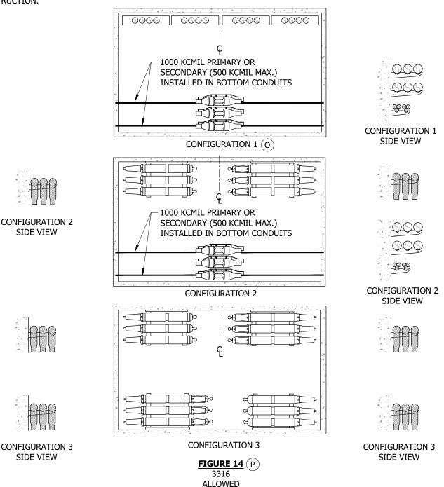
FOR ALL SIZES OF PRIMARY CABLES AND UP TO 500 KCMIL SECONDARY CABLES MAXIMUM PLAN VIEW
