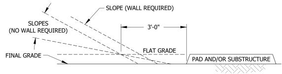
FIGURE 1 WHEN RETAINING WALLS ARE REQUIRED (A)
