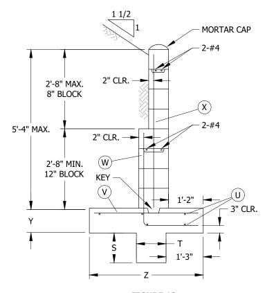
FIGURE 11 C-6 TYPICAL SECTION 3'-8" MAX.
