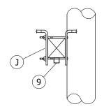
**DETAIL 1** FRONT VIEW CONDUIT WITH CABLE SUPPORT BRACKETS
