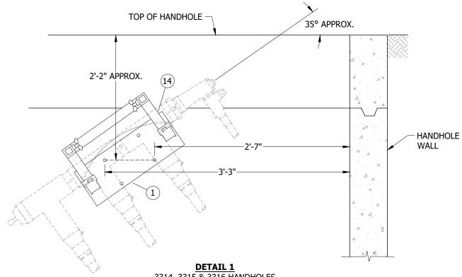
3314, 3315 & 3316 HANDHOLES TEE BRACKET ANGLE & INSTALLATION MEASUREMENTS FRONT VIEW
