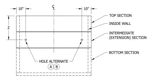
FIGURE 1 END VIEW OF HANDHOLE
