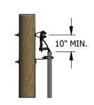
**FIGURE 4** SECONDARY AERIAL CABLE TANGENT CONSTRUCTION SIDE VIEW
