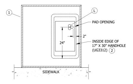
FIGURE 9 UG3512 INSTALLATION SINGLE-PHASE FUSE CABINET PLAN VIEW
