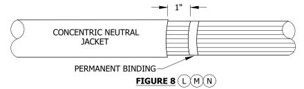
O APPLY A 2 INCH WIDE STRIP OF SEALING COMPOUND, 1 INCH OVER THE CONCENTRIC NEUTRAL JACKET AND 1 INCH OVER THE SEMICONDUCTING MATERIAL AND CONCENTRIC NEUTRALS. TIGHTLY PUSH THE SEALING COMPOUND AROUND THE CONCENTRIC NEUTRAL WIRES.
