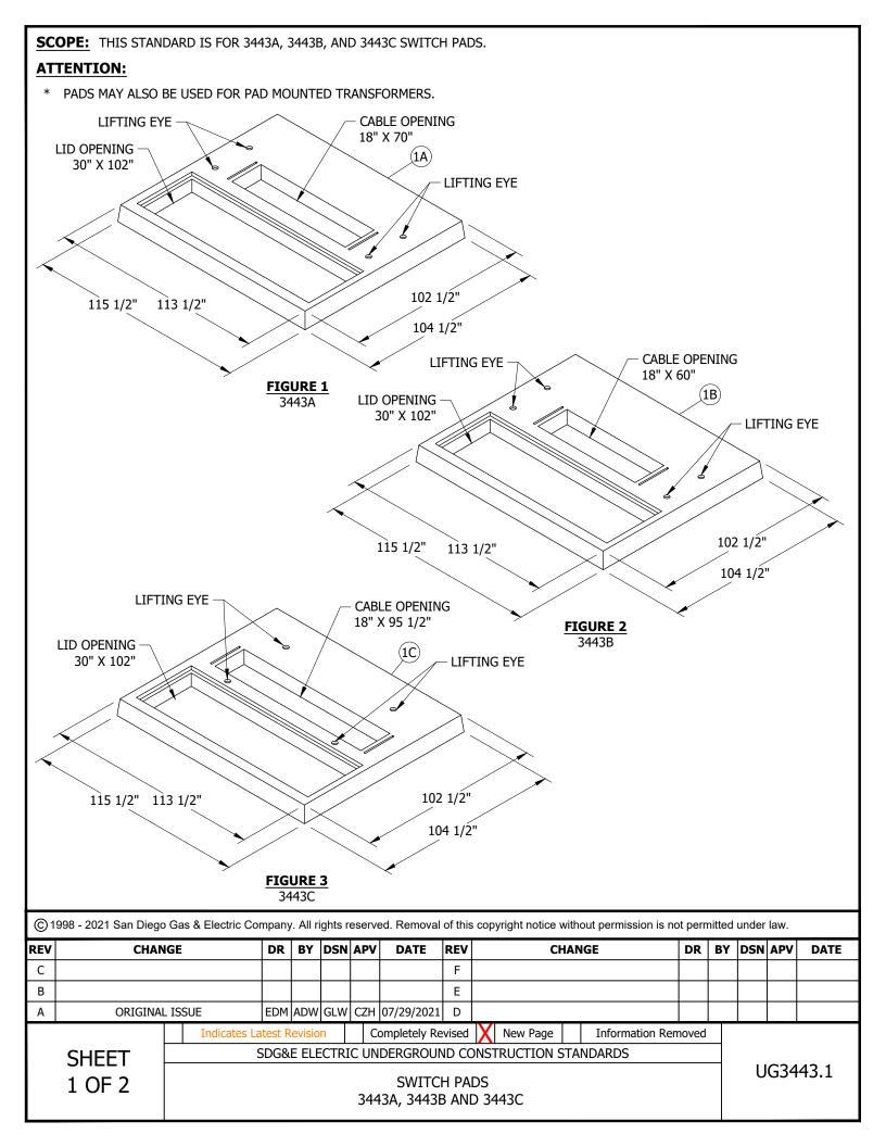
A. USE ALL FOUR LIFTING EYES WHEN MOVING PAD.
