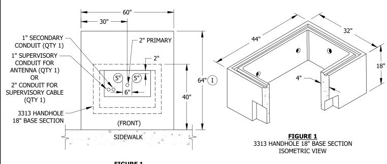
FIGURE 1 PAD FOR EATON-COOPER SERVICE RESTORER ( I ) PREFERRED INSTALLATION PLAN VIEW
