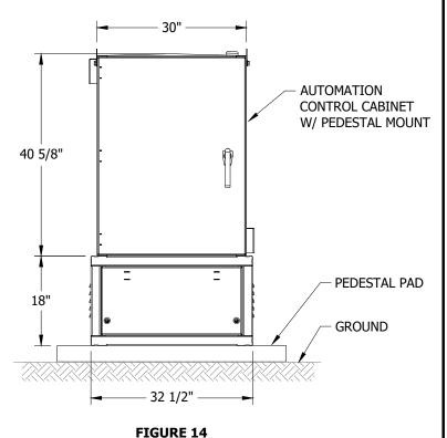
FOUR-WAY SUBMERSIBLE 600A SCADA 12KV W/ PEDESTAL SEE TABLE 6
