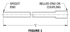
(PVC) POLYVINYLCHLORIDE CONDUIT CONDUIT STRAIGHT SECTIONS
