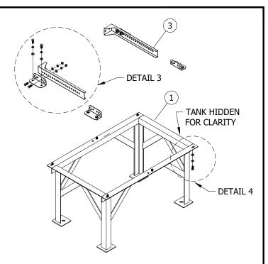
FOUR-WAY SUBMERSIBLE STAND (MANUAL & SCADA)
