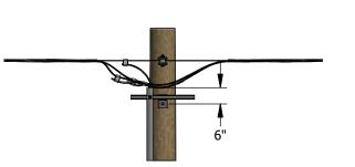
FIGURE 4 SECONDARY AERIAL CABLE TANGENT CONSTRUCTION FRONT VIEW
