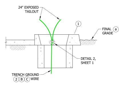
FIGURE 4 3416 PAD WITH 3311 HANDHOLE SECTION VIEW
