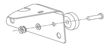
**FIGURE 4** ANTENNA BRACKET MAGNETIC MOUNTING KIT ASSEMBLY (A)
