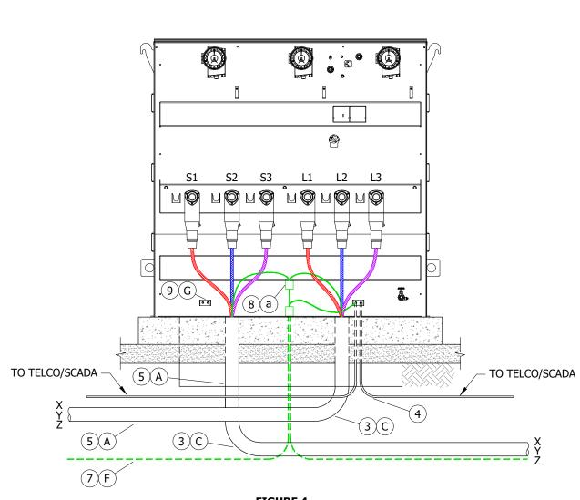
FIGURE 4 CABLE CONNECTION DIAGRAM **DELTA CONNECTED REGULATOR**
