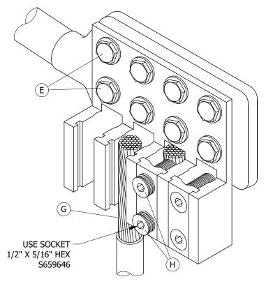
FIGURE 1 LAY-IN CONNECTOR
