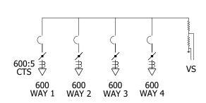
FOUR-WAY VAULT MOUNT 600A MANUAL/NON-SCADA
