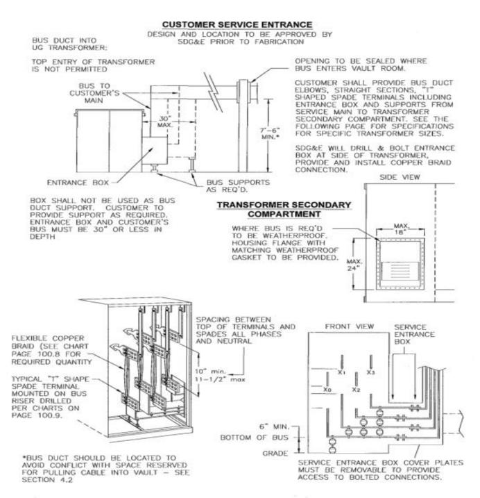
Figure 2 - Typical bus duct configuration for pad-mounted transformer.
