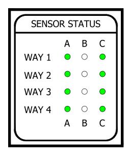
FIGURE 27 SUCCESSFUL CONNECTION TO THE LPCN NETWORK (A)
