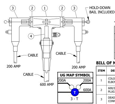
FIGURE 4 MANHOLE INSTALLATION SUBSURFACE CONNECTIONS 200 AND 600 AMP DEADBREAK
