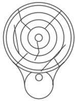
METHOD 1 IMPREGNATED FIBER CONDUIT OF 1/4" MINIMUM THICKNESS
