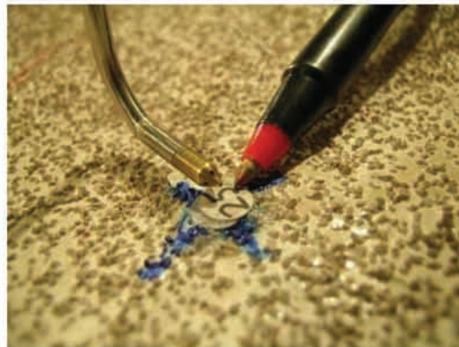
Exhibit 3c. Measurement probe to sample 3 components of velocity.
