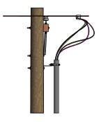
FIGURE 2 OPEN SECONDARY "AIR MAILING" SIDE VIEW
