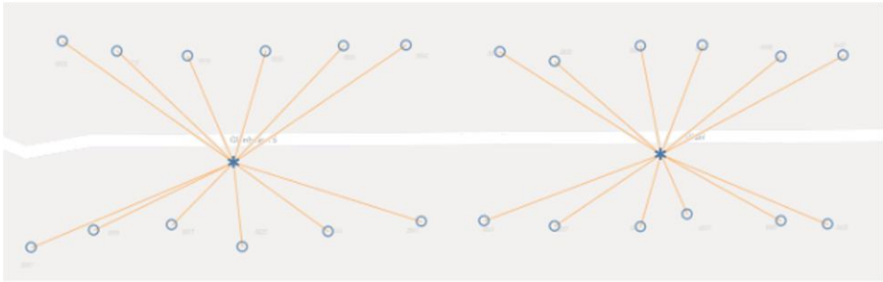
Figure 1. Typical meter-to-transformer connectivity on a suburban street
