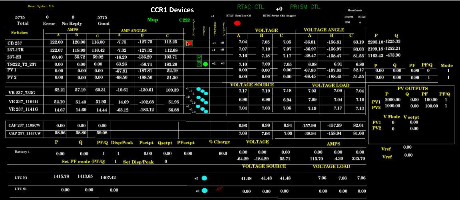
Figure 2-26. Snapshot of the master controller HMI (CCR1 – Baseline System 1)
