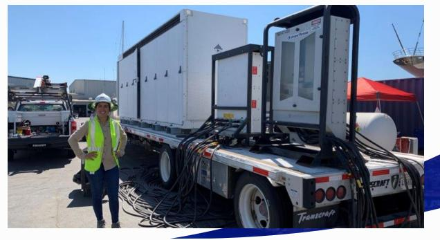
Mobile Battery Energy Storage Solution (MBESS)
